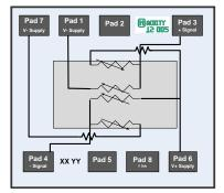
Schematic Layout of AC3010Pressu re Die
