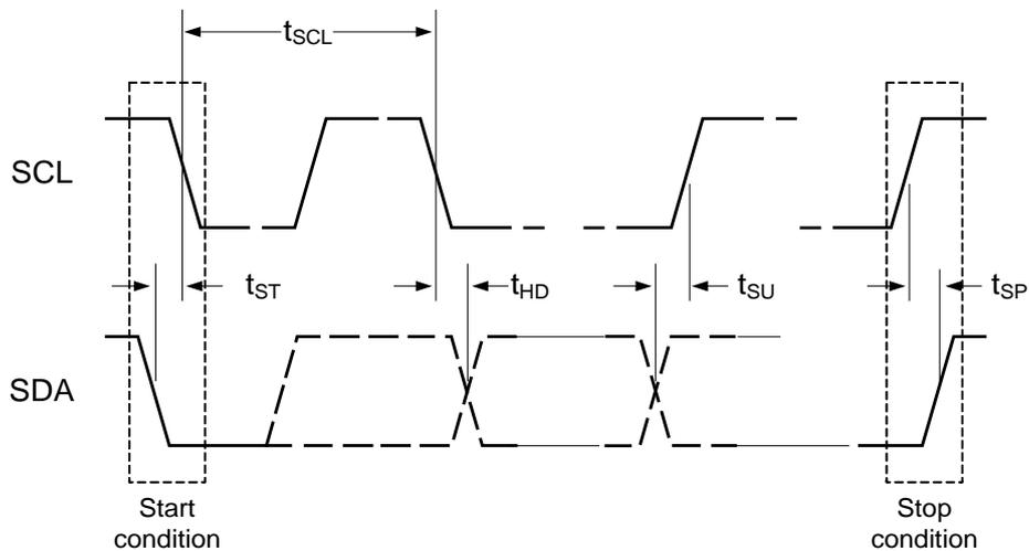
**Figure 2: I<sup>2</sup>C Data Transfer**
