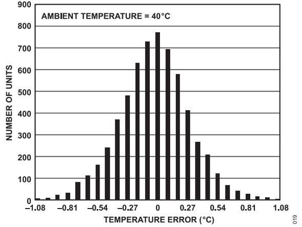
Figure 19. Ambient Temperature Error @ 3 V
