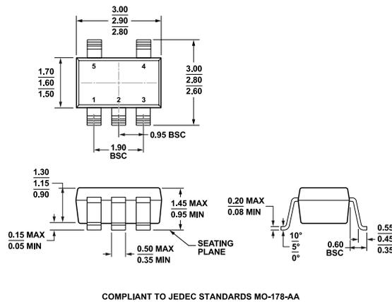
Figure 22. 5-Lead Small Outline Transistor Package [SOT-23] (RJ-5)
