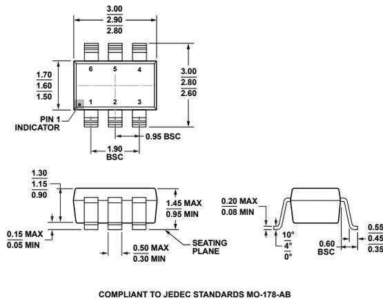
Figure 20. 6-Lead Small Outline Transistor Package [SOT-23] (RJ-6)
