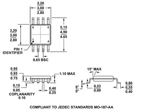
Figure 21. 8-Lead Mini Small Outline Package [MSOP] (RM-8)
