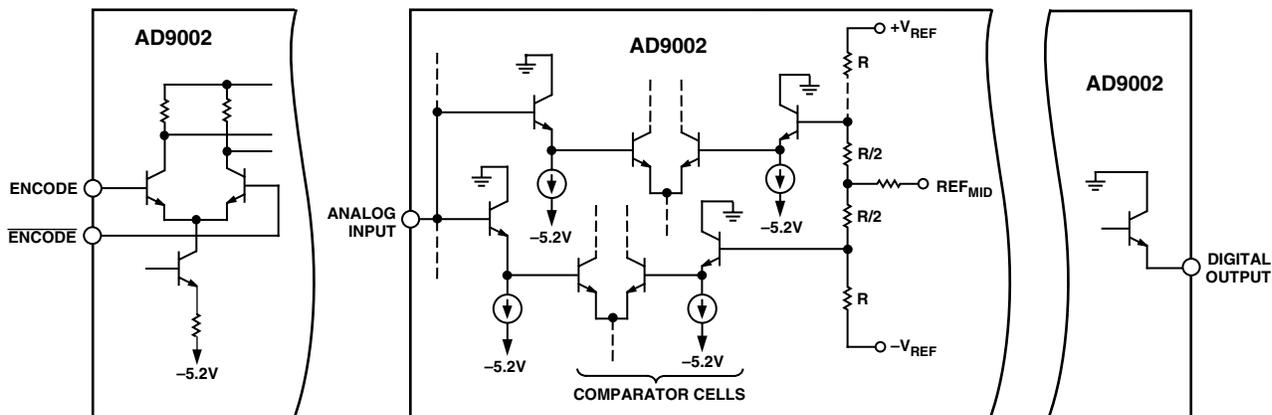
Figure 2. Input/Output Circuits
