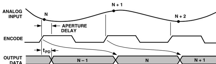
Figure 1. Timing Diagram
