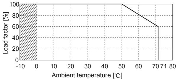
\*In case of ADA600F-24, load factor 100% means output 24V, 21A at ACIN100V, 24V, 25A at ACIN200V.
