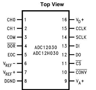
**Figure 1. 16-Pin Wide Body SOIC Package**
