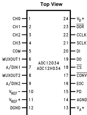
**Figure 3. 24-Pin Wide Body SOIC, PDIP, SSOP Packages**
