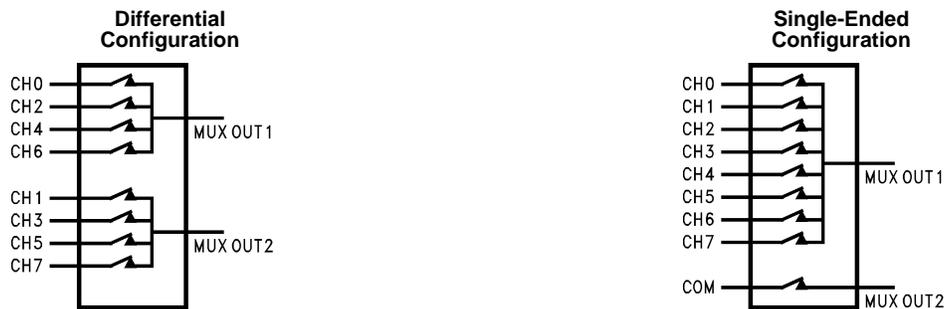
A/DIN1 and A/DIN2 can be assigned as the + or - input
