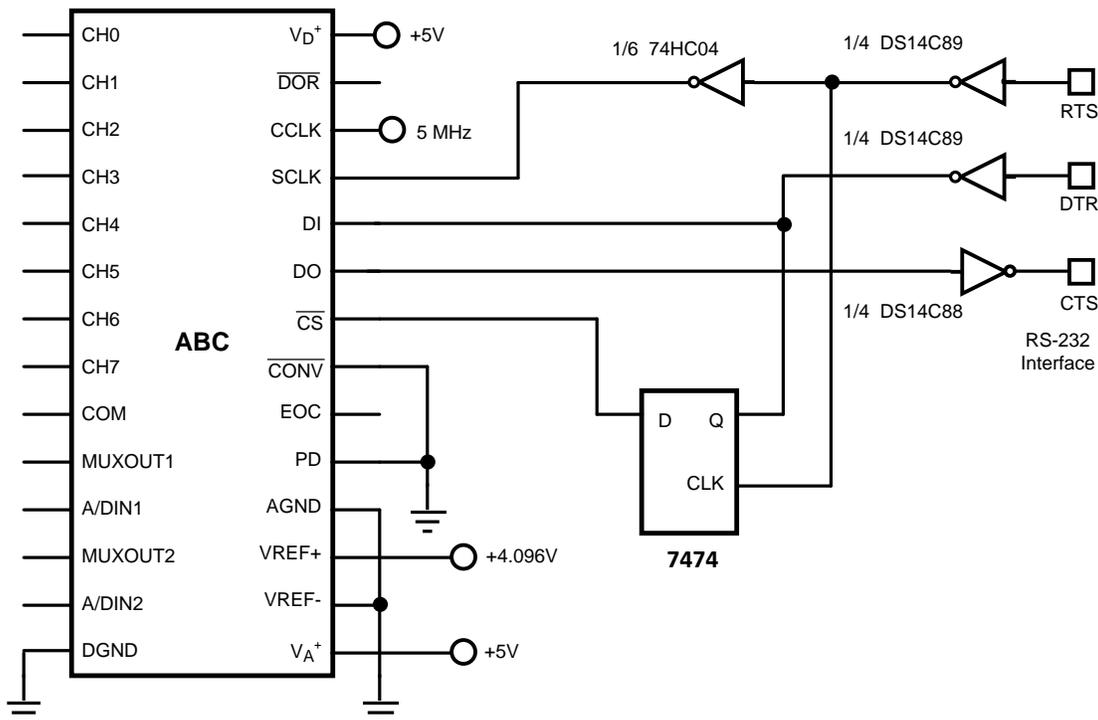
**Note:** V<sub>A</sub><sup>+</sup>, V<sub>D</sub><sup>+</sup>, and V<sub>REF</sub><sup>+</sup> on the ADC12038 each have 0.01 μF and 0.1 μF chip caps, and 10 μF tantalum caps. All logic devices are bypassed with 0.1 μF caps.
