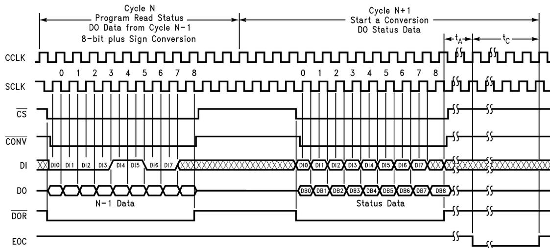
**Note:** In order for all 9 bits of Status Information to be accessible, the last conversion programmed before Cycle N needs to have a resolution of 8 bits plus sign, 12 bits, 12 bits plus sign, or greater.
