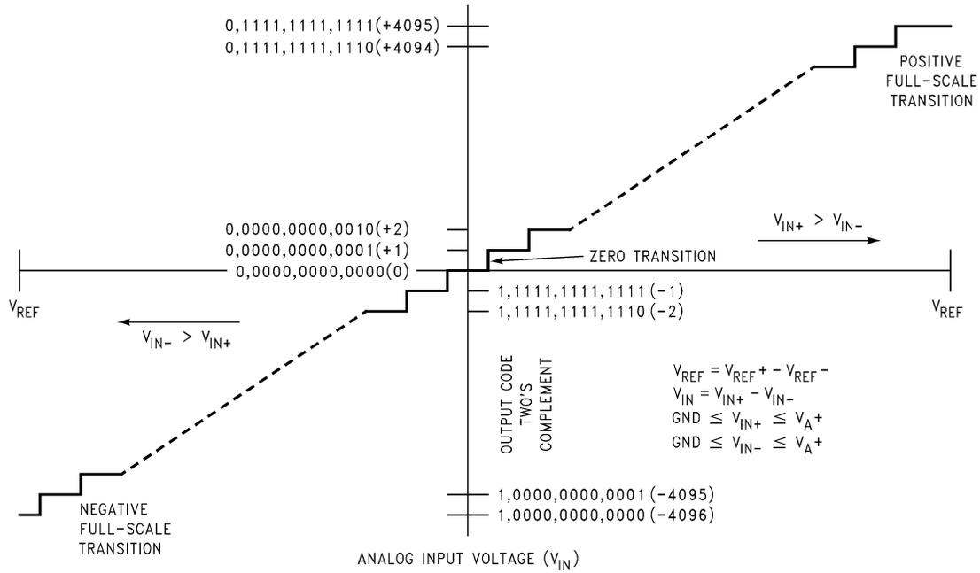
Figure 5. Transfer Characteristic
