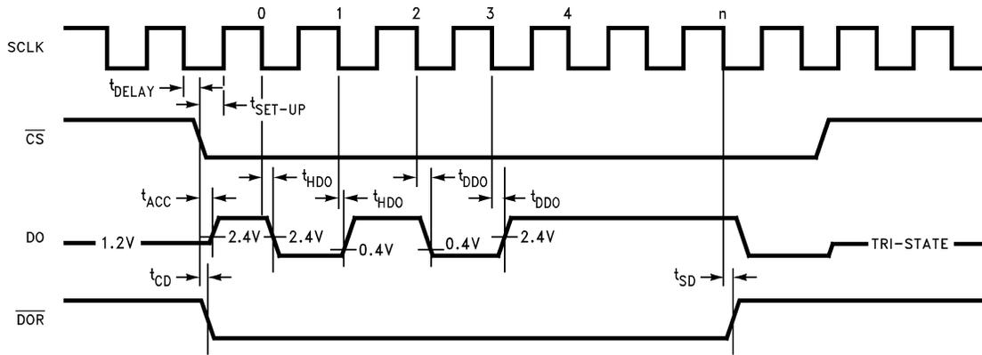
Figure 46. DO Data Output Timing Using  $\overline{CS}$
