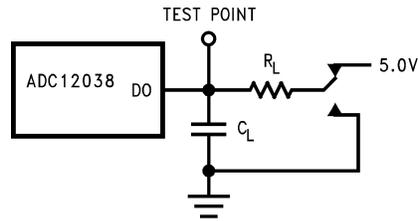
Figure 40. DO “TRI-STATE” ( $t_{1H}$ ,  $t_{0H}$ )
