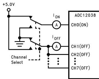
Figure 42. Leakage Current
