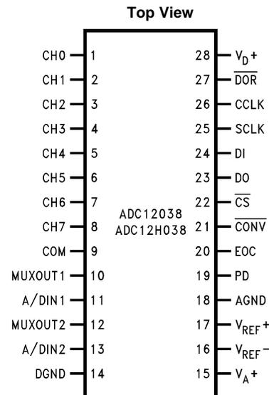
**Figure 4. 28-Pin Wide Body SOIC Package**
