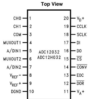
**Figure 2. 20-Pin Wide Body SOIC Package**
