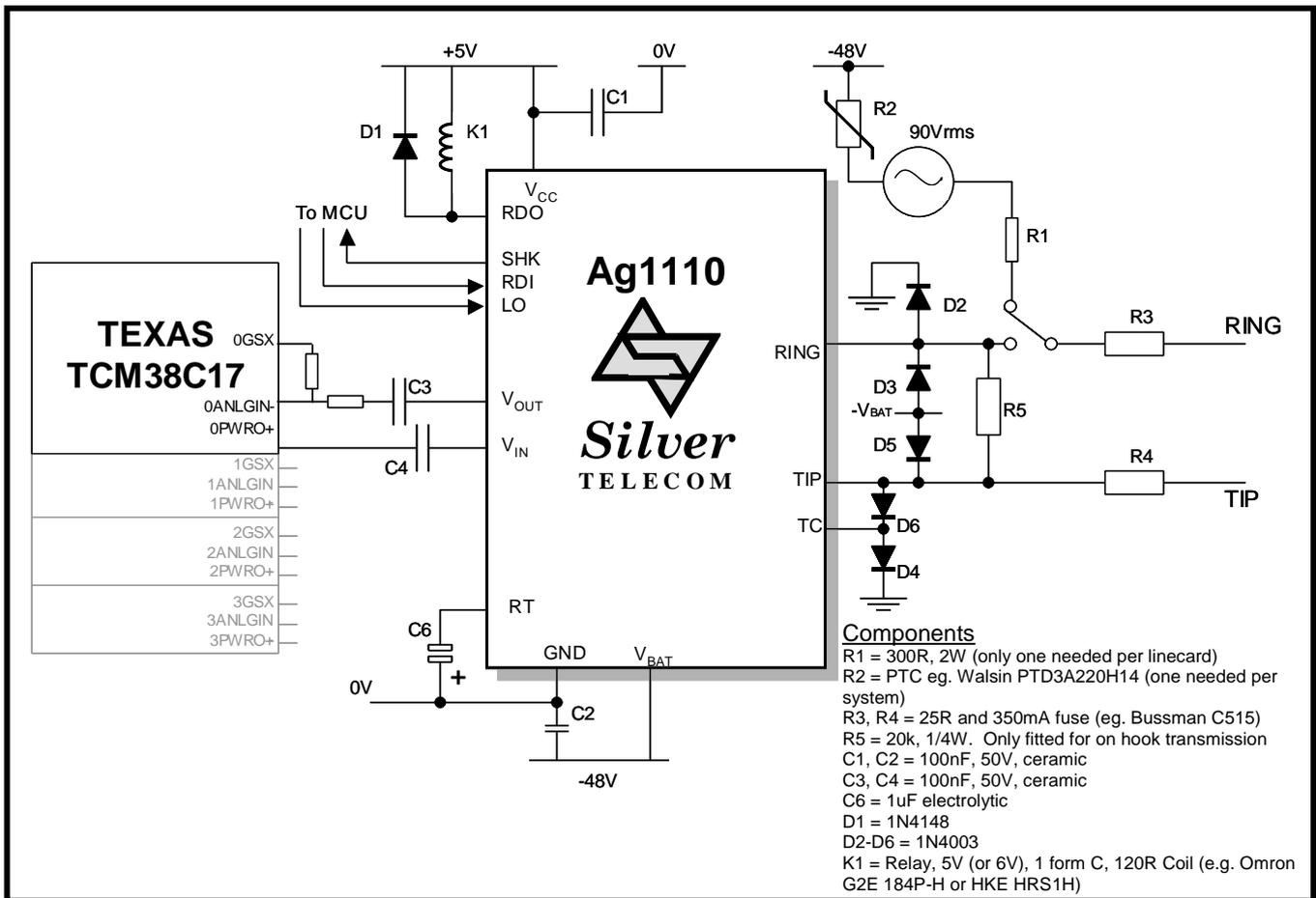
**Figure 5: Ringing Application Diagram with Codec**
