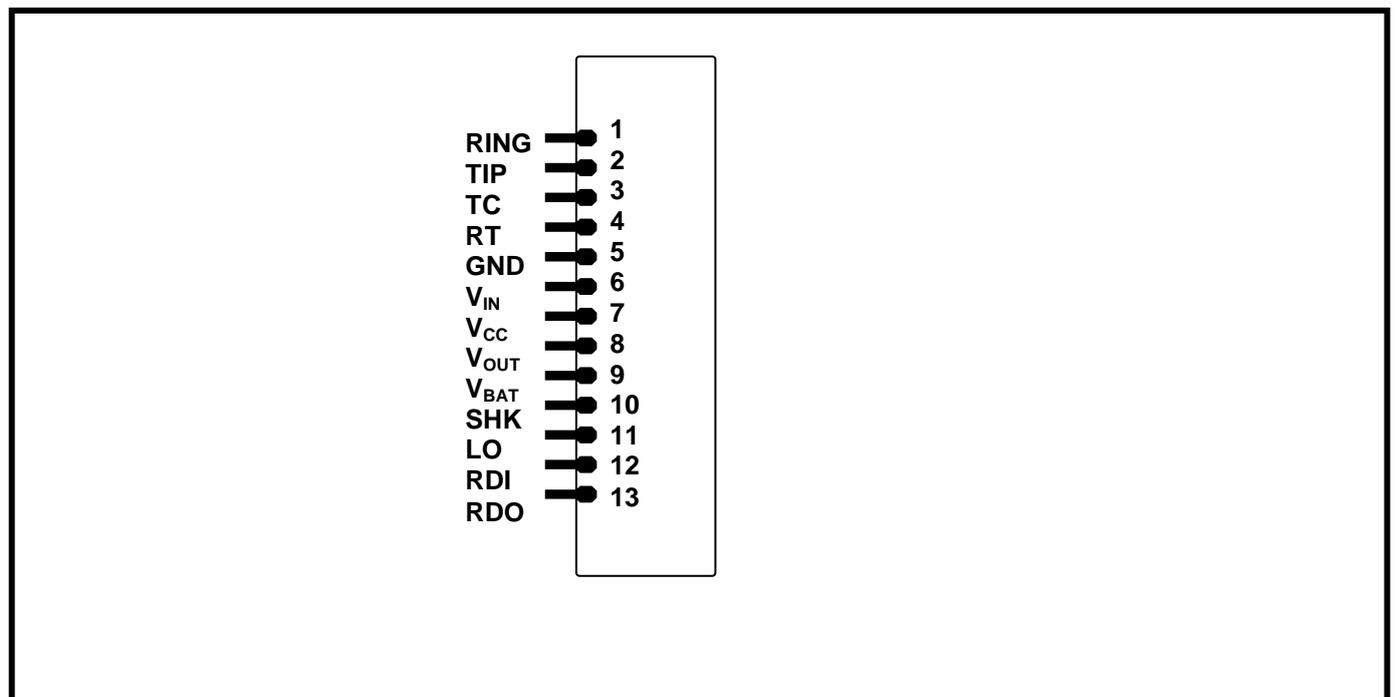
**Figure 4: Pin Connections**
