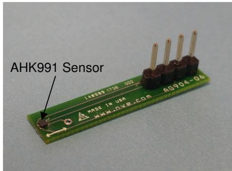
**Figure 2. AHK991 on a circuit board.**
