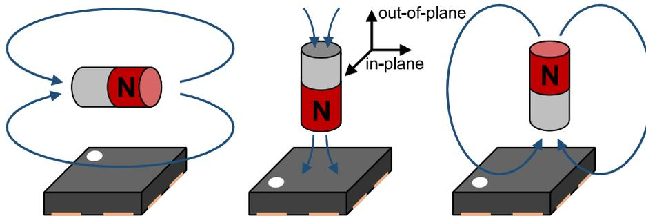
**Figure 1. AHK991 sensor direction of magnetic sensitivity.**
