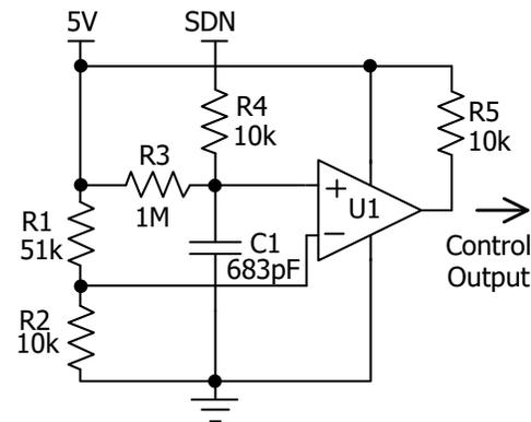
Figure 6. The Equivalent Circuit for SDN Port
