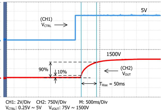
Figure 12. Rising Trail for Large Signal Response
