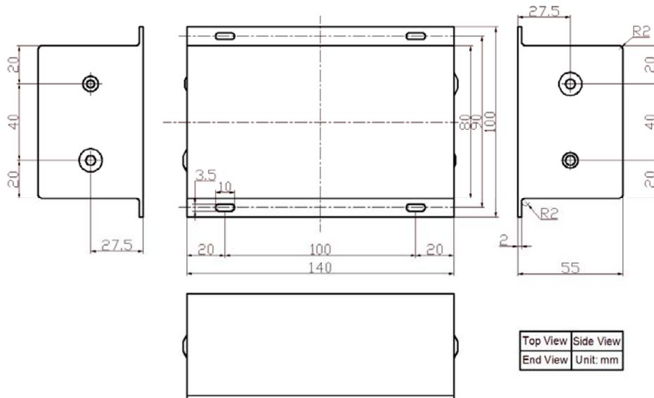
Figure 11. Dimensions for AHV24VN15KV1MAW
