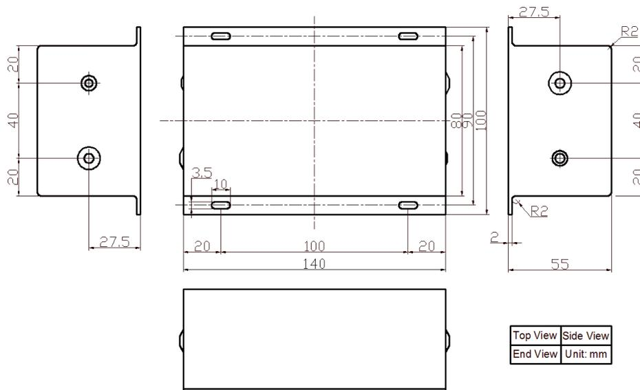
Figure 11. Dimensions for AHV24VN30KV2R5MAW
