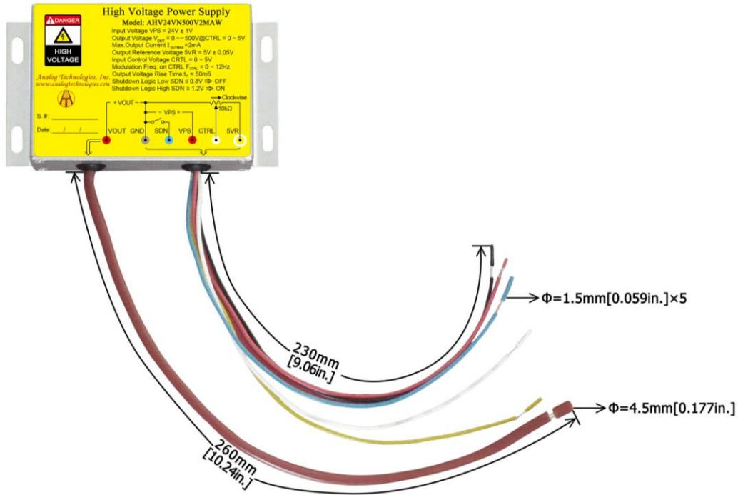
Figure 13. Connecting Lead Wires of AHV24VN500V5MAW
