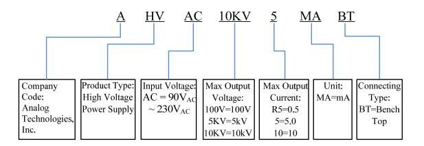
Figure 5. Naming rules of AHVAC10KV5MABT
