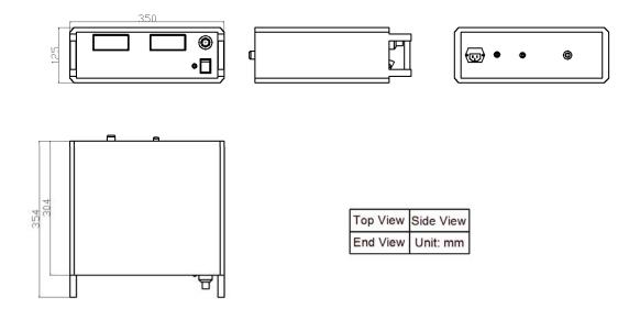
Figure 7. Dimensions for AHVAC10KV5MABT
