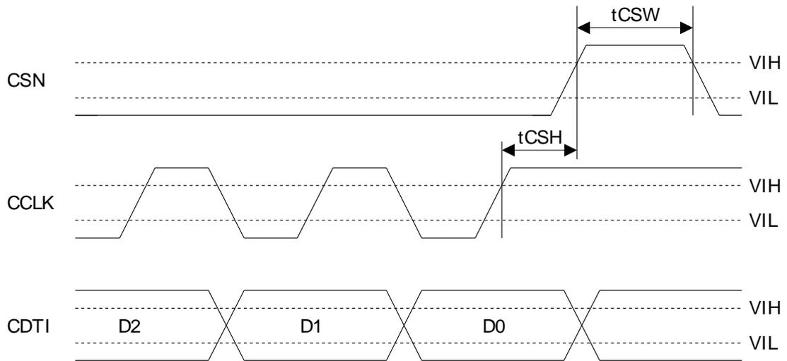
Figure 14. WRITE Data Input Timing (CSP pin = "L")
