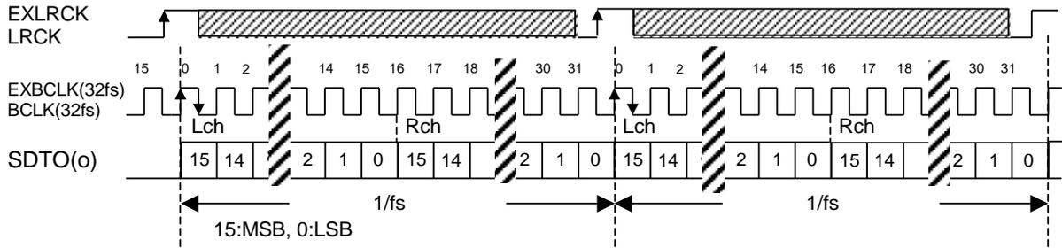
Figure 26. Mode 0 Timing (BCKP = "0", MSBS = "0", M/S = "0" or "1")
