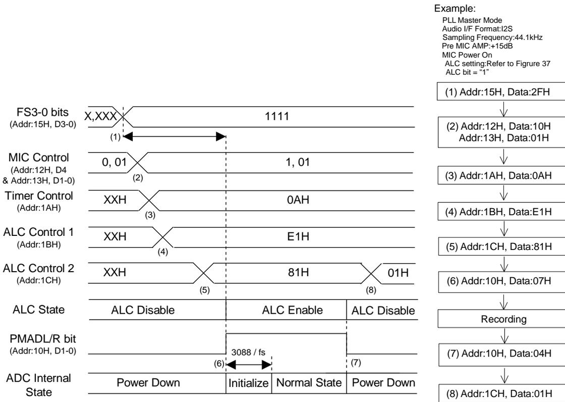
Figure 52. MIC Input Recording Sequence
