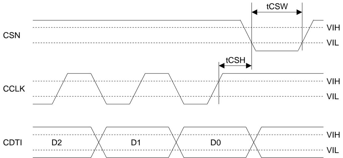
Figure 16. WRITE Data Input Timing (CSP pin = "H")
