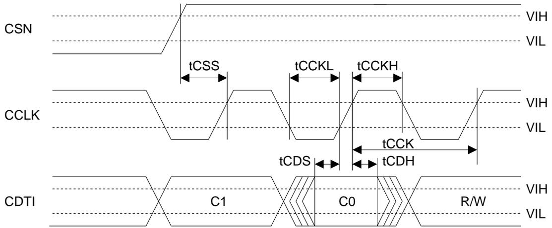
Figure 15. WRITE Command Input Timing (CSP pin = "H")
