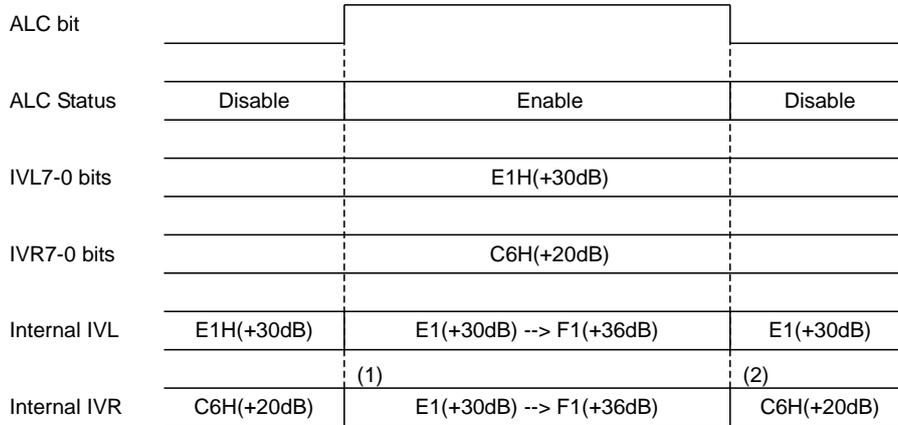
Figure 40. IVOL value during ALC operation
