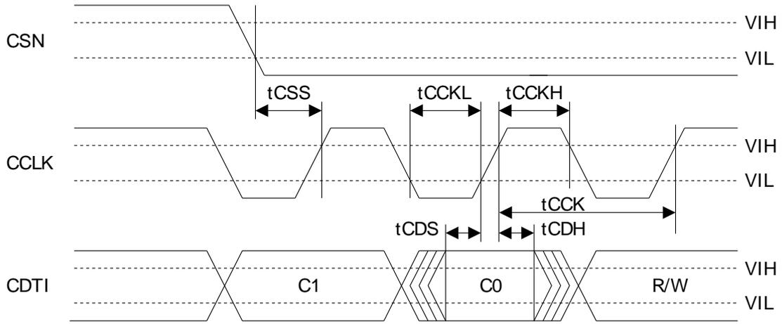
Figure 13. WRITE Command Input Timing (CSP pin = "L")
