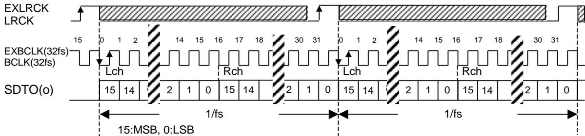
Figure 29. Mode 0 Timing (BCKP = "1", MSBS = "1", M/S = "0" or "1")
