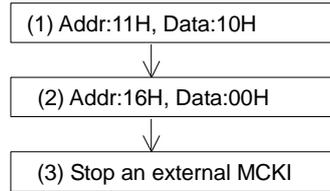
Figure 53. Clock Stopping Sequence (1)
