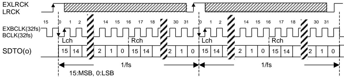
Figure 27. Mode 0 Timing (BCKP = "1", MSBS = "0", M/S = "0" or "1")
