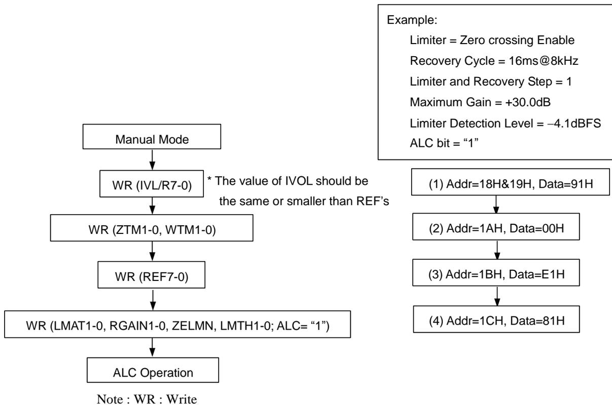
Figure 39. Registers set-up sequence at ALC operation
