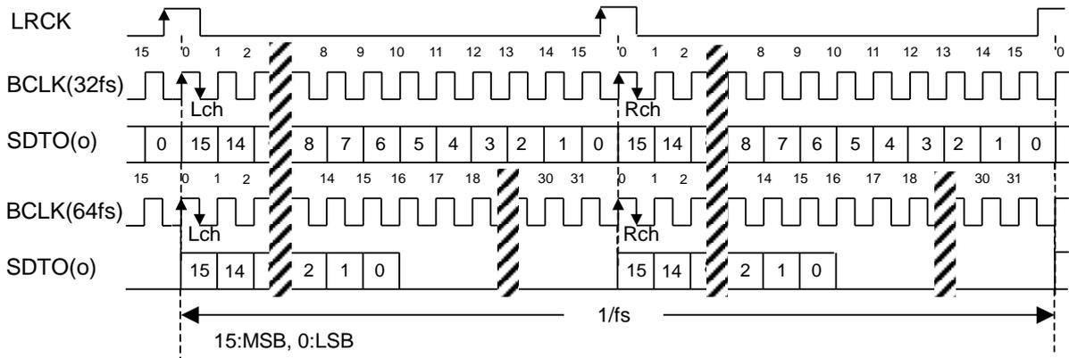
Figure 30. Mode 1 Timing (BCKP = "0", MSBS = "0", M/S = "1")
