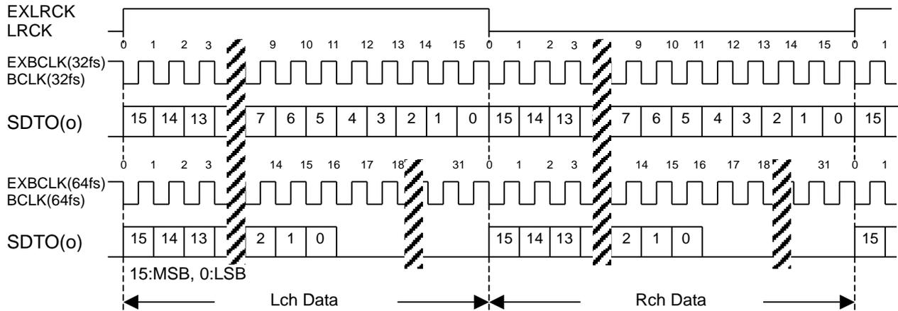
Figure 34. Mode 2 Timing (MSB justified, M/S = “0” or “1”)
