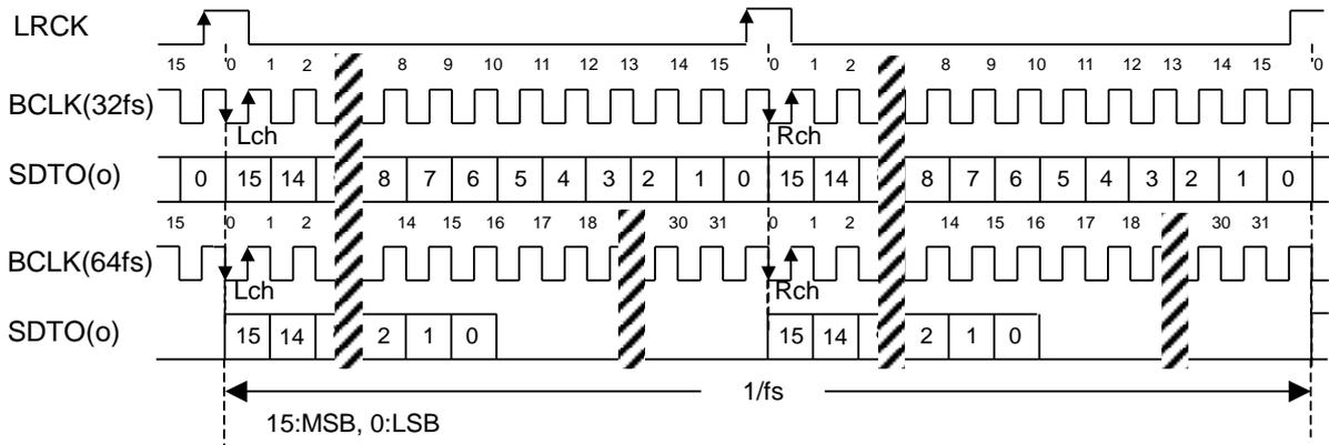
Figure 31. Mode 1 Timing (BCKP = "1", MSBS = "0", M/S = "1")
