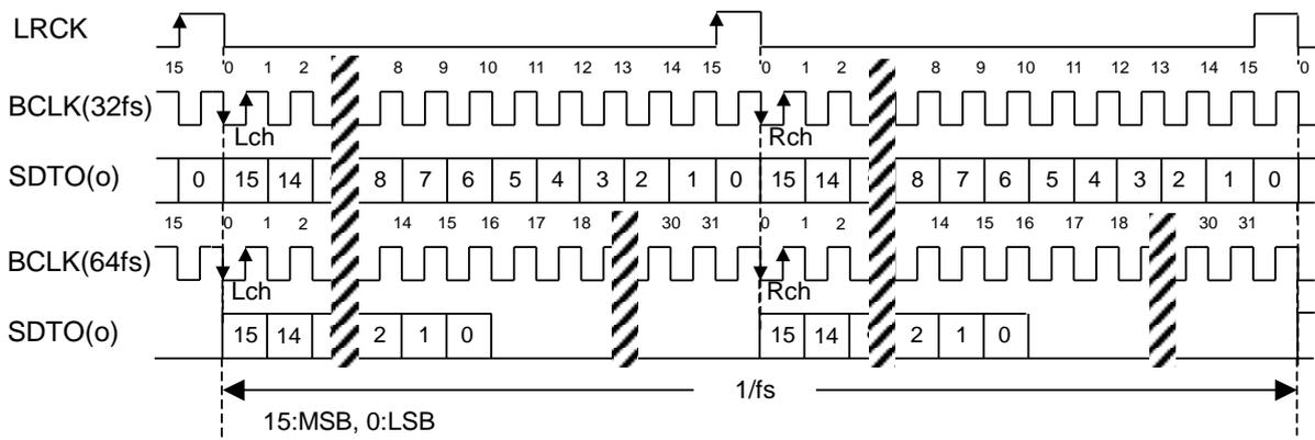
Figure 33. Mode 1 Timing (BCKP = "1", MSBS = "1", M/S = "1")
