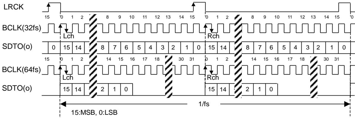
Figure 32. Mode 1 Timing (BCKP = "0", MSBS = "1", M/S = "1")
