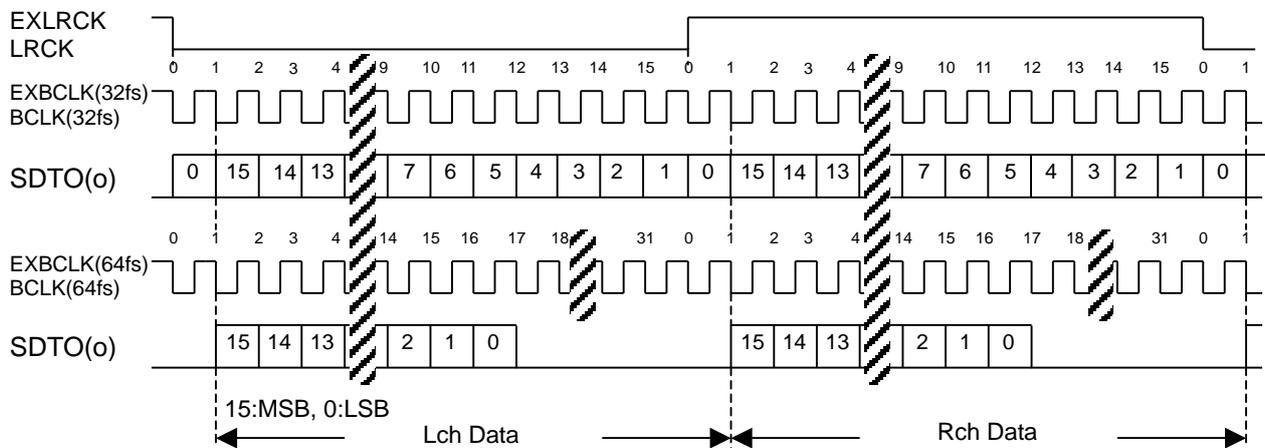
Figure 35. Mode 3 Timing (I<sup>2</sup>S, M/S = “0” or “1”)
