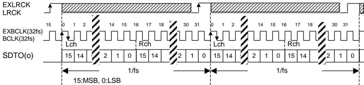
Figure 28. Mode 0 Timing (BCKP = "0", MSBS = "1", M/S = "0" or "1")
