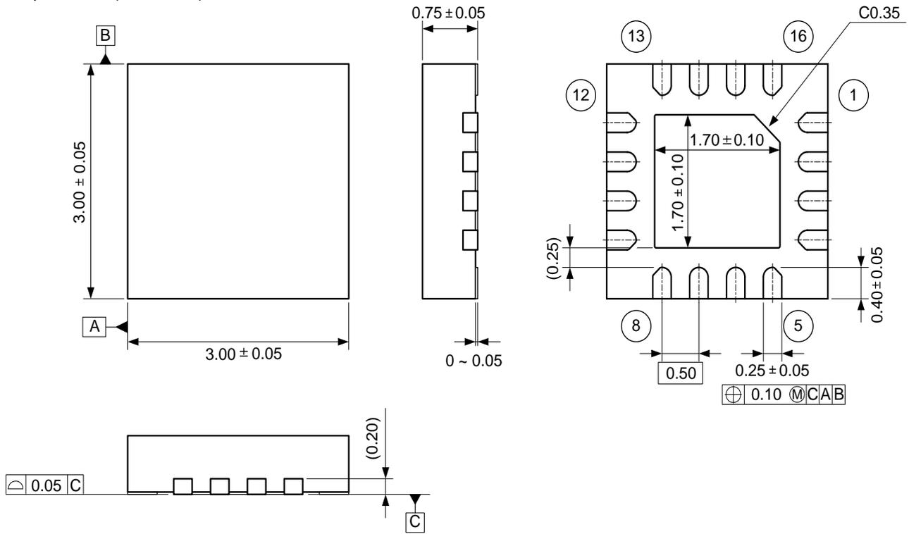
\* The exposed pad on the bottom surface of the package must be open or connected to the ground.
