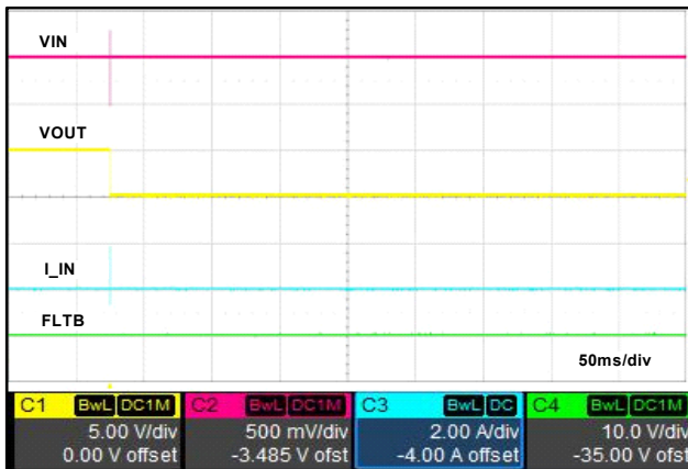
Figure 15. Short Circuit Protection (No Load, Device Option -04)
