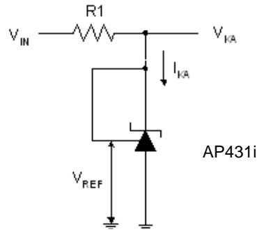
Test Circuit 4 for  $V_{KA} = V_{REF}$
