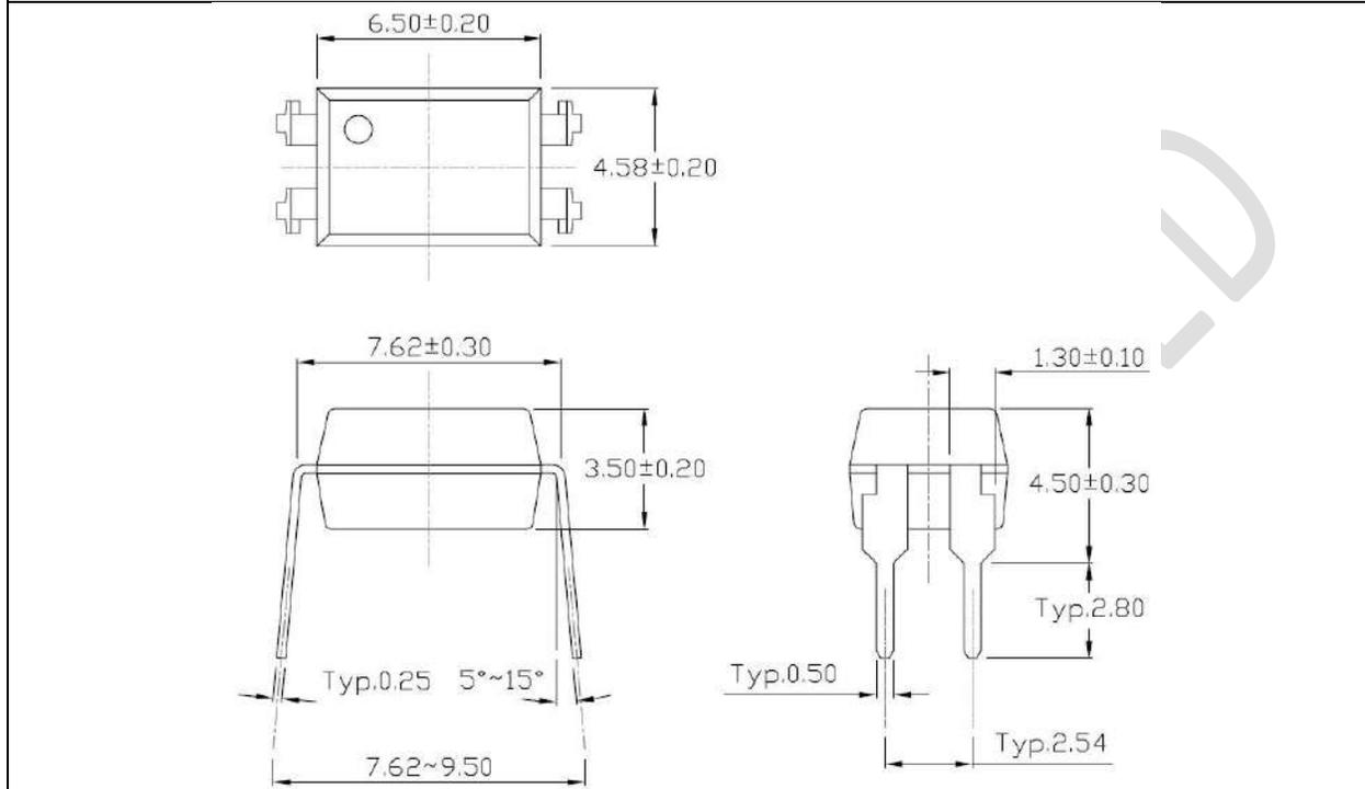
**Gullwing (400mil) Lead Forming – Through Hole (M Type) – APC-817xx-M**
