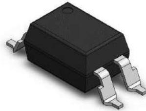
The APC-817 series combines an AlGaAs infrared emitting diode as the emitter which is optically coupled to a silicon planar phototransistor detector in a plastic DIP4 package with different lead forming options.
