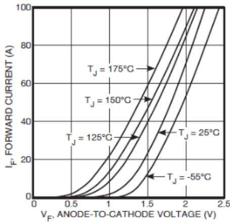
Figure 2 • Forward Current vs. Forward Voltage
