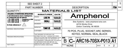
70 POS, PLUG, SOCKET,ARC SERIES,KEYED, NORMAL SEAL,BLACK DMG NO: ARC16-70SX-P013
