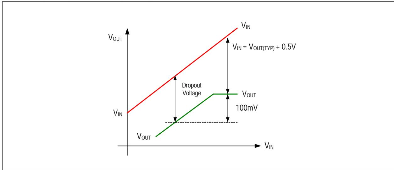
Figure 15 shows the variation of  $V_{OUT}$  as  $V_{IN}$  is varied for a certain load current. The practical value of dropout is the differential voltage ( $V_{OUT} - V_{IN}$ ) measured at the point where the LDO output voltage has fallen by 100mV below the nominal, fully regulated output value. The nominal regulated output voltage of the LDO is that obtained when there is 500mV (or greater) input-output voltage differential.
