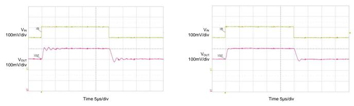
Figure 4. Test Result Without RNULL
