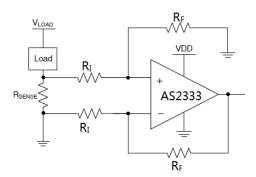
Figure 8. Low-Side Current Monitor Application
