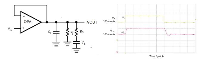
Figure 6. Circuit with Snubber Circuit
