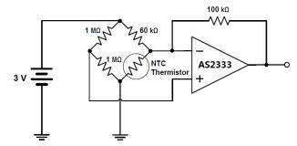
Figure 9. Bridge Circuit Amplification
