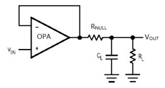
Figure 3. Capacitive Load with R<sub>NULL</sub>
