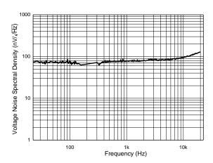
Figure 1. Input Voltage Noise in Conventional Amplifier (AZV832)
