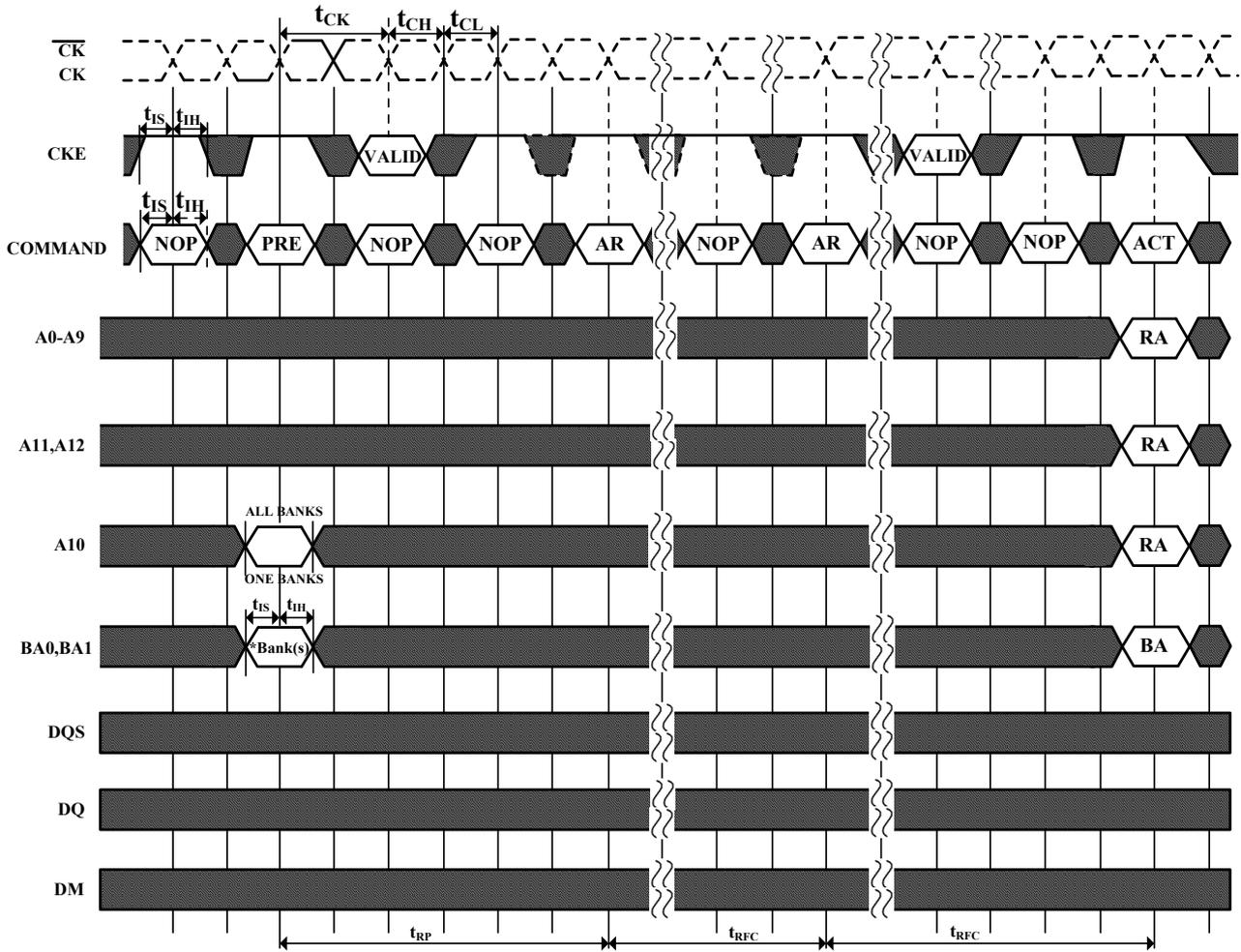
\* = "Don't Care", if A10 is HIGH at this point; A10 must be HIGH if more than one bank is active (i.e., must precharge all active banks)
