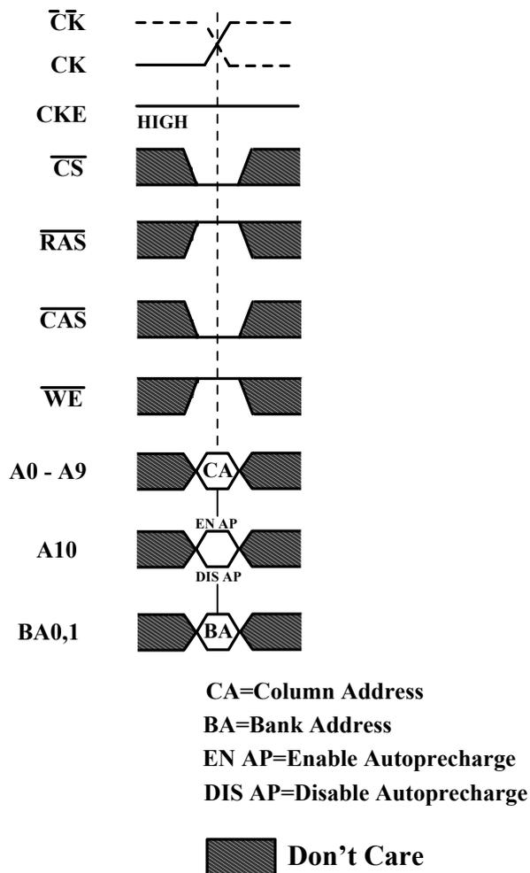
**Figure 9. Read Burst Required CAS Latencies (CL=2)**
