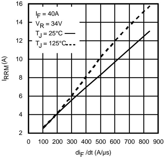
**Fig. 18** - Typical Recovery Current vs. di/dt
