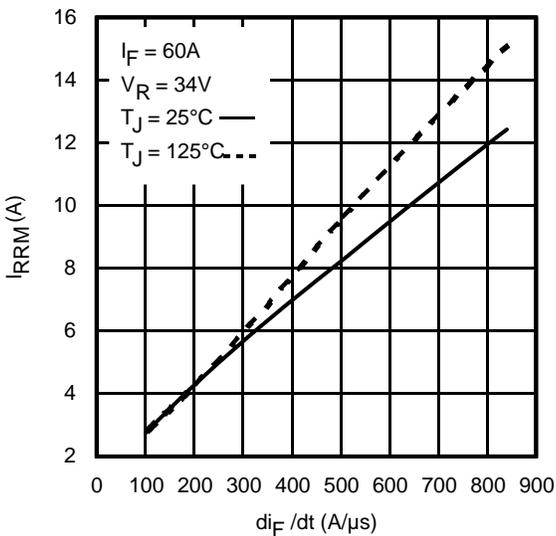
**Fig. 20** - Typical Recovery Current vs. di/dt
