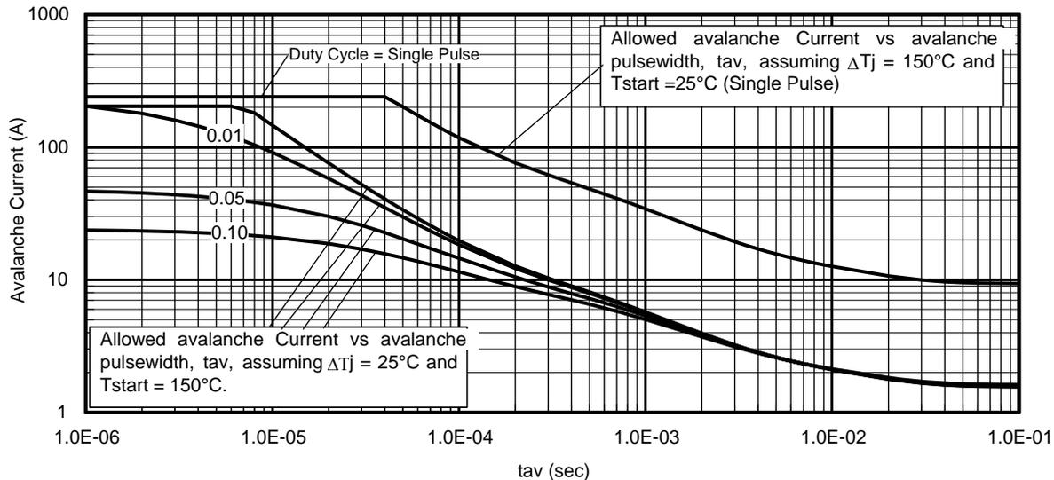
**Fig 14. Typical Avalanche Current vs. Pulse width**
