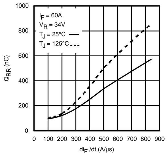
**Fig. 21** - Typical Stored Charge vs. di/dt
