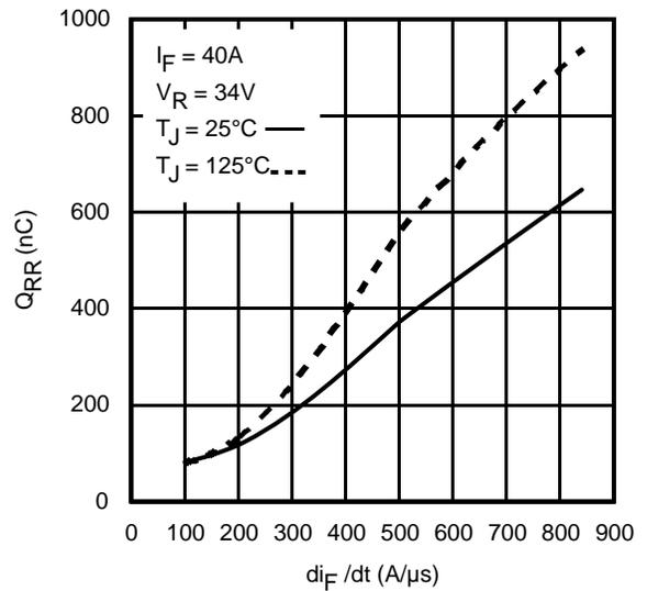
**Fig. 19** - Typical Stored Charge vs. di/dt
