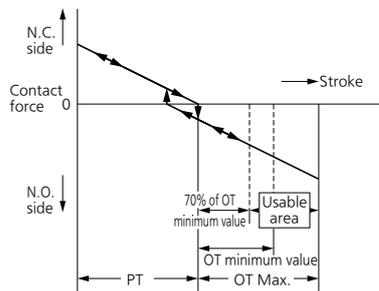
In addition, even if FS type switch actuator is pushed to full limit of operating position, it does not affect product life. However, heavy impact and excessive loading should not be applied.
