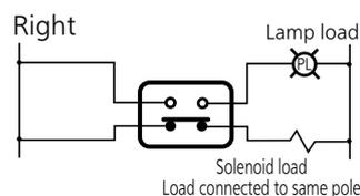
Example of wrong power supply connection (connection to different poles of power supply)
