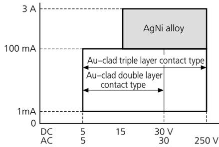
Note) If the contact is being used in the constant low-level circuit load range, the Au-clad double layer contact type is recommended. If there is a danger of the current being less than 0.5 A, for instance if the contact is being turned on and off, the Au-clad triple layer contact type is recommended.
