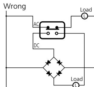
3) Avoid circuits which apply voltage between contacts. (This may lead to mixed deposition.)
