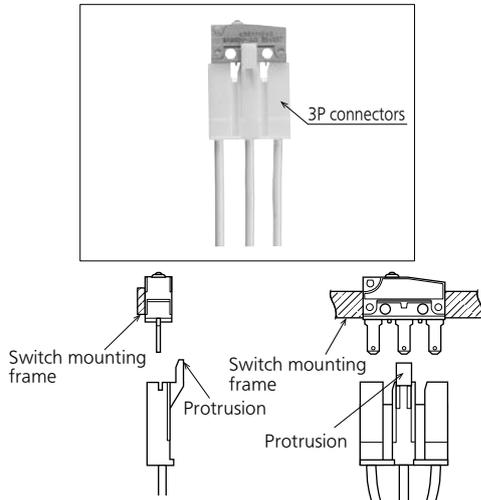
As shown in the diagram, the protrusion on the 3P connector can only be inserted on the corresponding side of the mounting frame. That is, using the plunger as a reference, the subminiature switches can only be inserted in the direction shown in the diagram: it is not possible to mount it the wrong way round.
