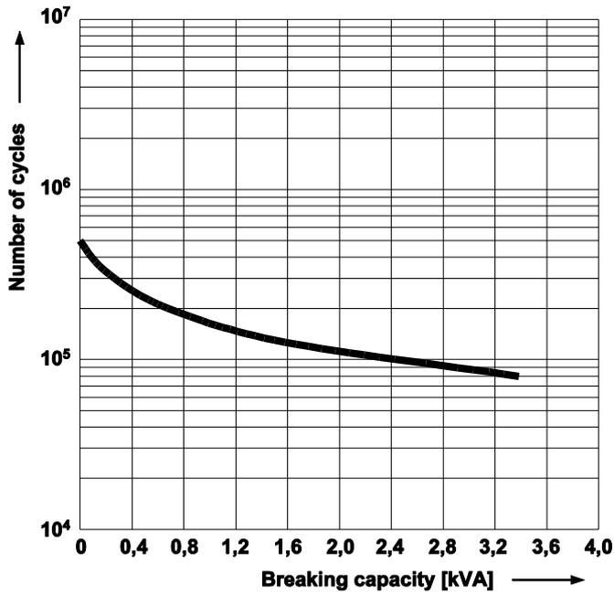
Electrical life reduction factor at inductive AC load
