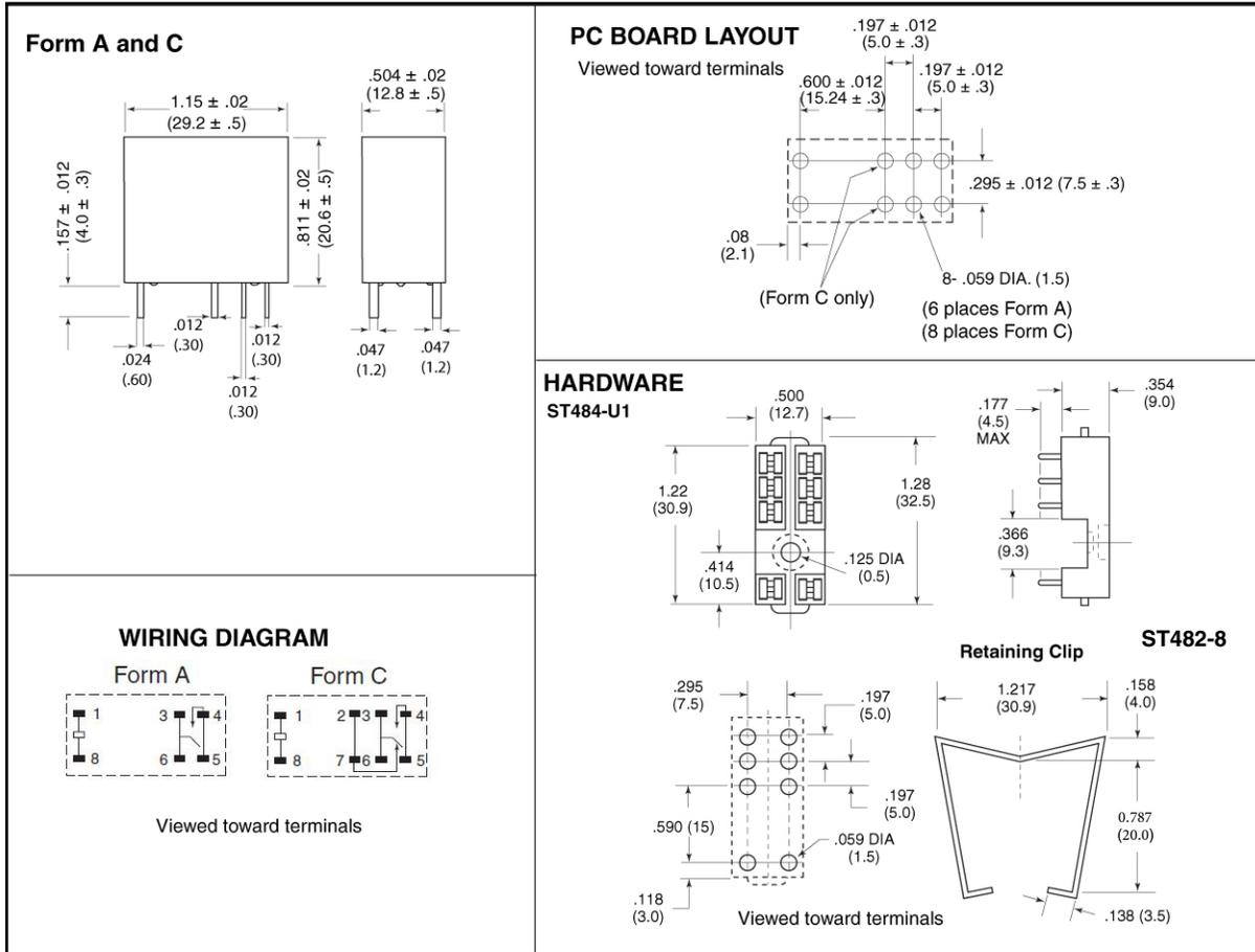
Dimensions in inches with metric equivalents in parentheses. Tolerance:  $\pm .010$ " unless specified.
