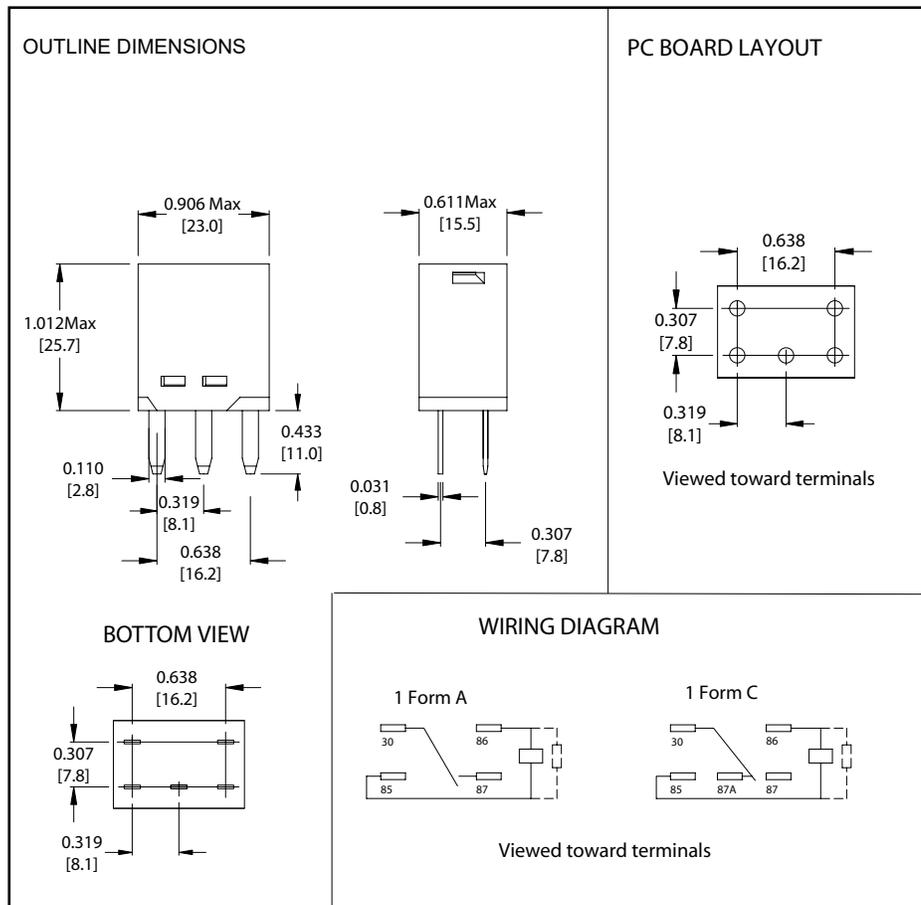
Dimensions in inches with metric equivalents in parentheses. Tolerance:  $\pm .010$ "
