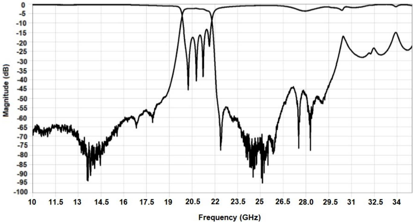
\*Typical de-embedded measured performance mounted on a connectorized test fixture. DEB is 0.010in RO4350B with 50.0Ohm CPW ground traces going into the ports at room temperature.
