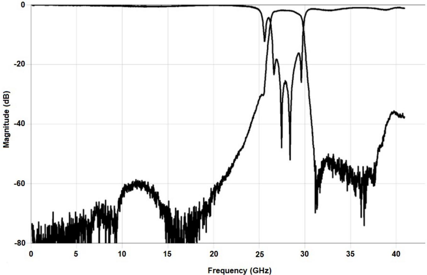
\*Typical de-embedded measured performance mounted on a connectorized test fixture. DEB is 0.010in RO4350B with 50.0Ohm CPW ground traces going into the ports at room temperature.
