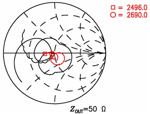
Figure 5: Reflection coefficient at output port.
