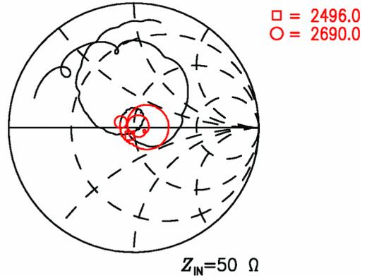
Figure 4: Reflection coefficient at input port.
