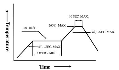
3. DIP soldering (Wave Soldering):
