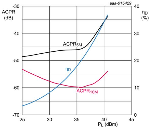
$T_{case} = 25\text{ }^{\circ}\text{C}$ ;  $V_{DS} = 28\text{ V}$ ;  $I_{Dq1} = 30\text{ mA}$ ;  $I_{Dq2} = 120\text{ mA}$ ;  $f = 900\text{ MHz}$ ; 1-carrier W-CDMA; test model 1; PAR = 9.9 dB at 0.01 % probability on CCDF. Per section.
