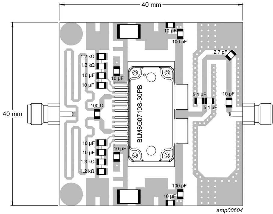
Printed-Circuit Board (PCB): Rogers 4350; thickness = 0.508 mm.
