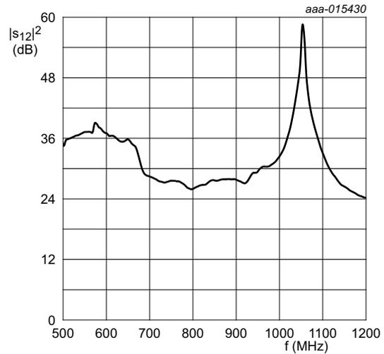
$T_{case} = 25\text{ }^{\circ}\text{C}$ ;  $V_{DS} = 28\text{ V}$ ;  $I_{Dq1} = 30\text{ mA}$ ;  $I_{Dq2} = 120\text{ mA}$ ; measured on evaluation board.
