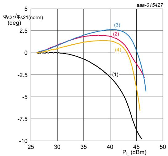
Normalized at  $P_L = 26\text{ dBm}$ ;  $T_{case} = 25\text{ }^\circ\text{C}$ ;  $V_{DS} = 28\text{ V}$ ;  $I_{Dq1} = 30\text{ mA}$ ;  $I_{Dq2} = 120\text{ mA}$ . Per section.
