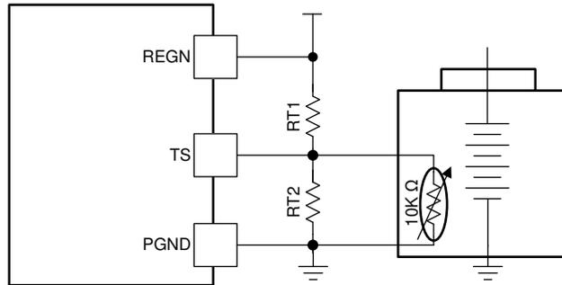
Assuming a 103AT NTC thermistor on the battery pack as shown above, the value of RT1 and RT2 can be determined by:
