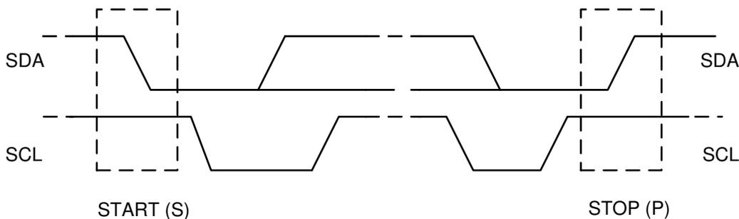
**Figure 7-8. START and STOP Conditions on the I<sup>2</sup>C Bus**
