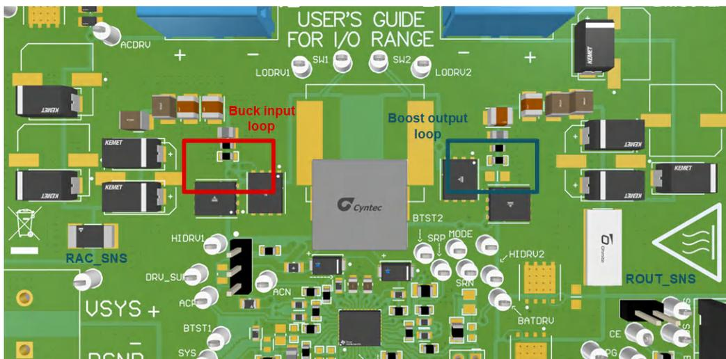
**Figure 10-1. PCB Layout Reference Example Top View**
