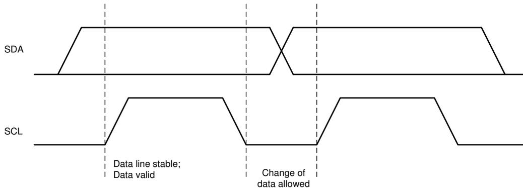
**Figure 7-7. Bit Transfers on the I<sup>2</sup>C Bus**
