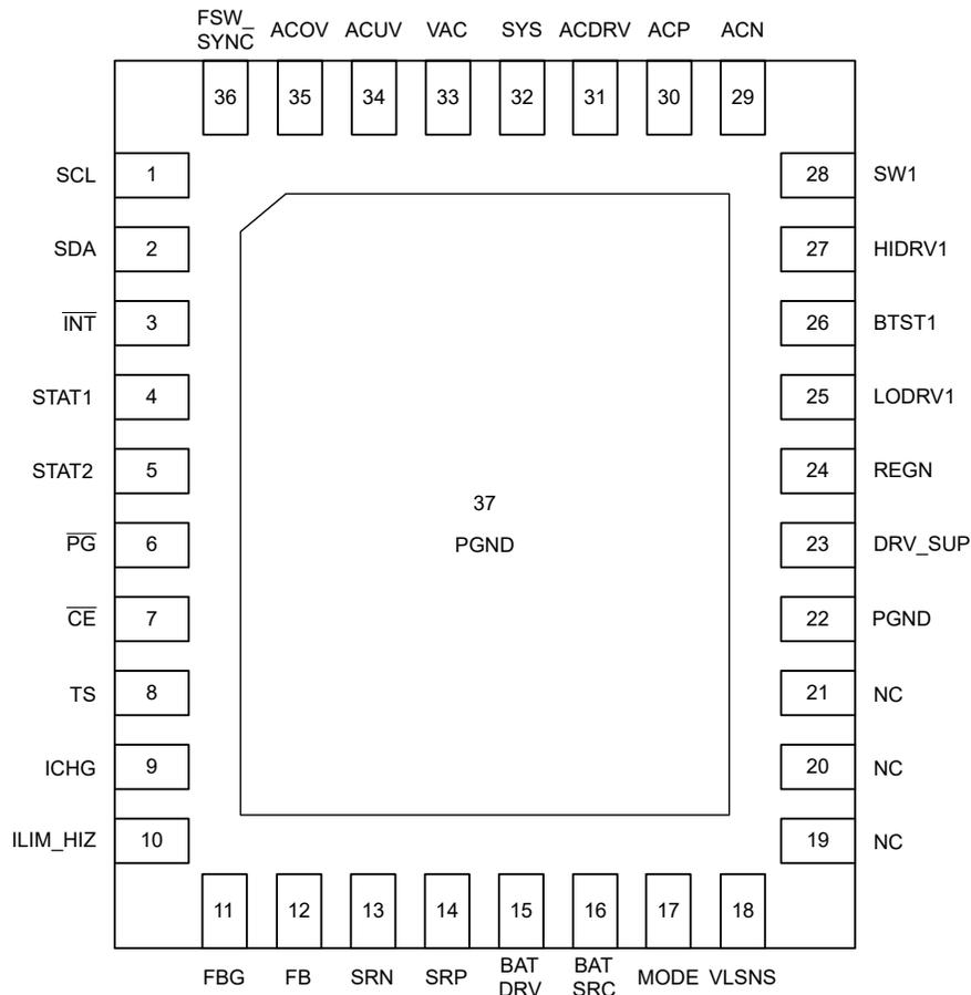
Figure 5-1. BQ25820, RRV Package 36-pin VQFN Top View
