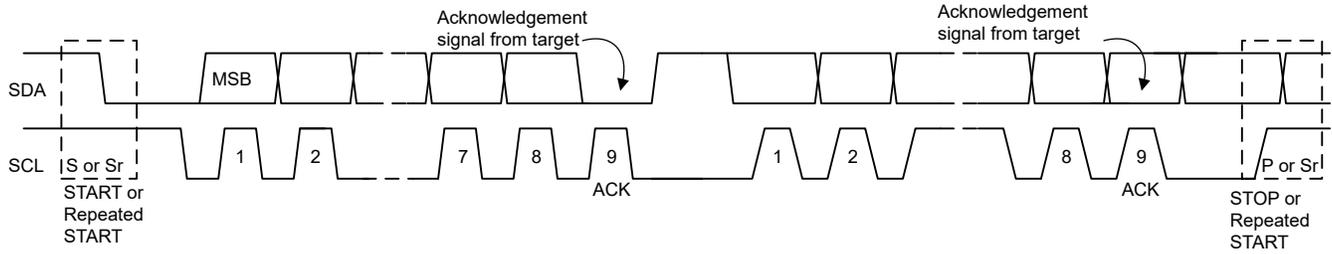
Figure 7-9. Data Transfer on the I<sup>2</sup>C Bus
