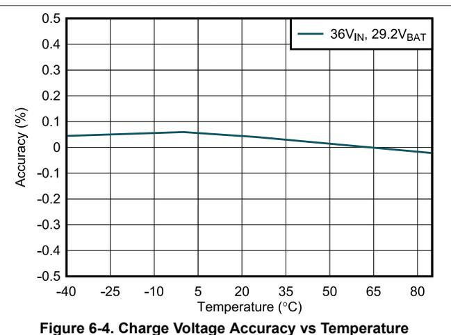
**Figure 6-4. Charge Voltage Accuracy vs Temperature**
