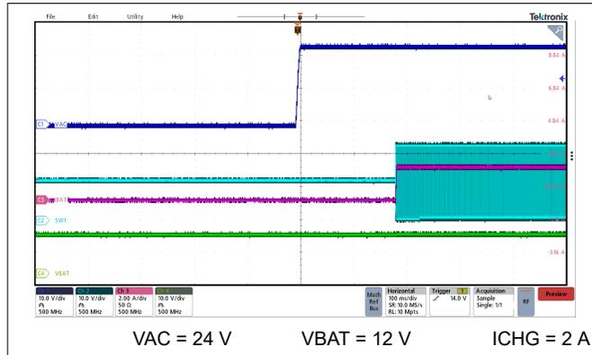
**Figure 8-3. VAC Plug-In Power Up with 2-A ICHG**
