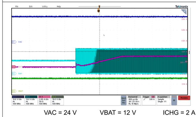
**Figure 8-5. Charge Enable via I<sup>2</sup>C with 2-A ICHG**
