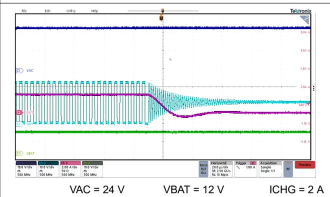
**Figure 8-6. Charge Disable via I<sup>2</sup>C with 2-A ICHG**
