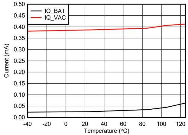
$I_{Q\_BAT}: VAC = 0 \text{ V}$     $I_{Q\_VAC}: VAC = 28 \text{ V}$     $EN\_HIZ = 1$
