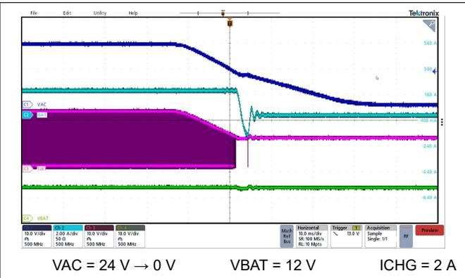
**Figure 8-4. VAC Un-plug Power Down with 2-A ICHG**
