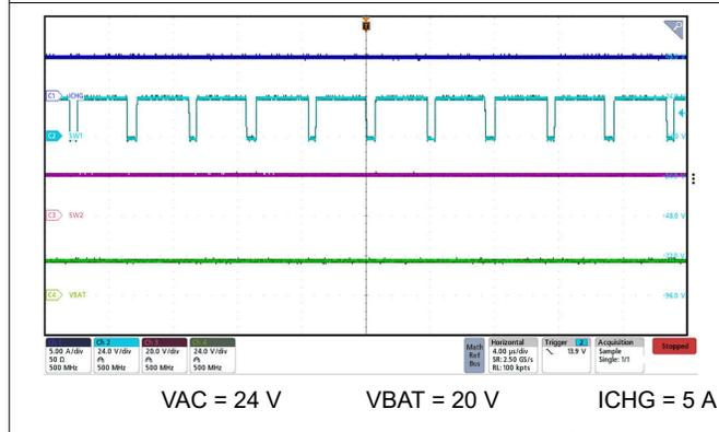
**Figure 8-7. Buck Switching Waveform**
