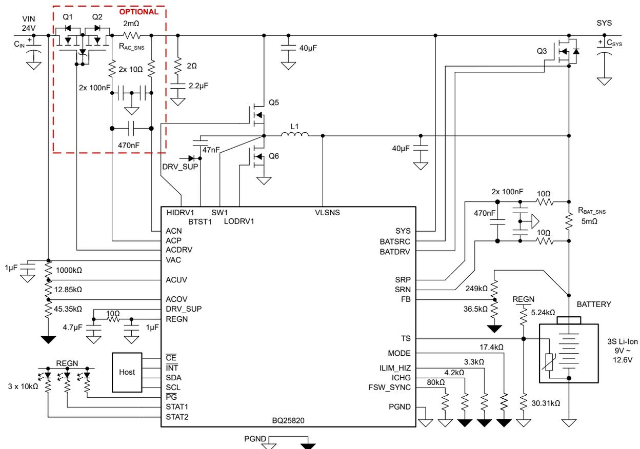
**Figure 8-1. BQ25820: I<sup>2</sup>C Controlled, 24 VAC with 3-S Li-Ion Battery, 10-A Charge Current and 350-kHz Switching Frequency**
