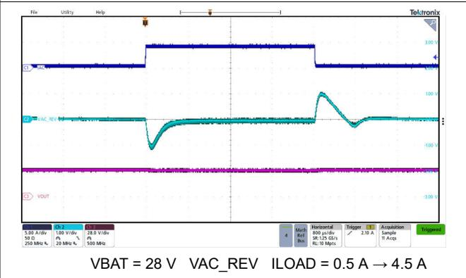
**Figure 8-8. Reverse Mode Boost Transient Reponse**
