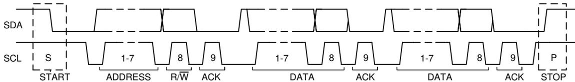
Figure 7-10. Complete Data Transfer on the I<sup>2</sup>C Bus
