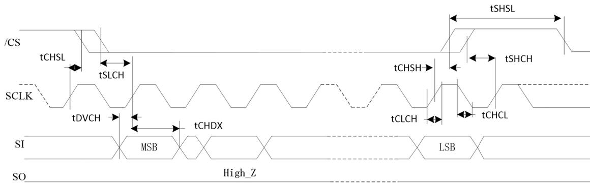
**Figure 24. Output Timing**
