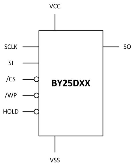
**Figure 2.** Pin Configuration SOP8 150/208 mil, TSSOP 173mil
