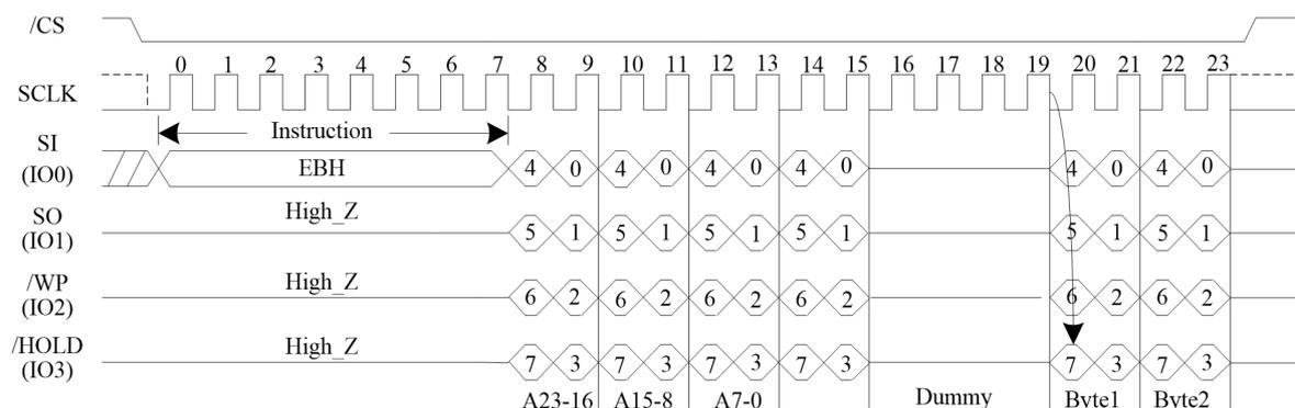
**Figure 17. Quad I/O Fast Read Sequence Diagram (Previous command set (M5-4)=(1,0))**
