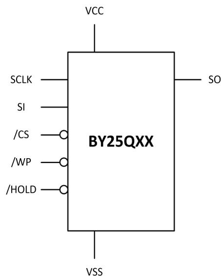
**Figure 2.** Pin Configuration SOP8
