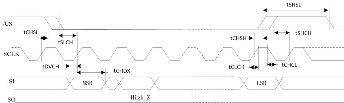
**Figure 47. Output Timing**
