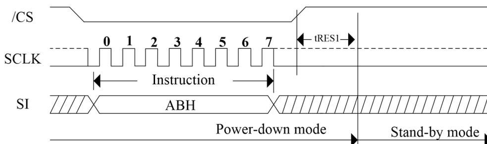
**Figure 28.** Release Power-Down/Read Device ID Sequence Diagram
