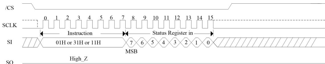
**Figure 8.b.** Write Status Register Sequence Diagram (QPI mode)
