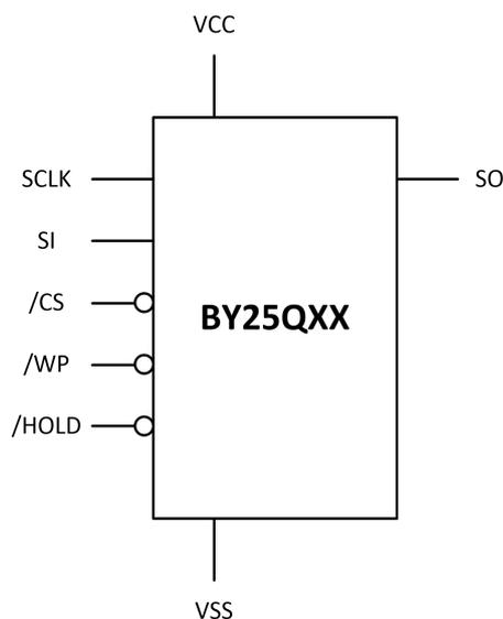
**Figure 2.** Pin Configuration SOP8
