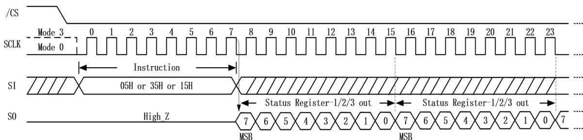
**Figure 7.b.** Read Status Register Sequence Diagram (QPI Mode)
