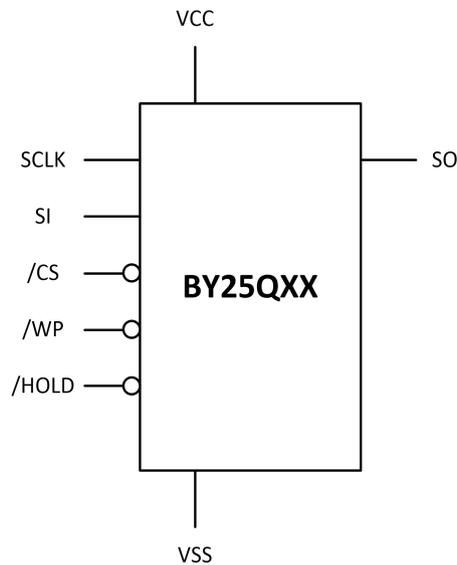
**Figure 2.** Pin Configuration SOP8
