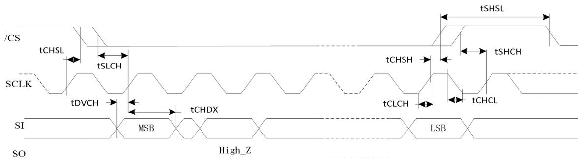
**Figure 47. Output Timing**
