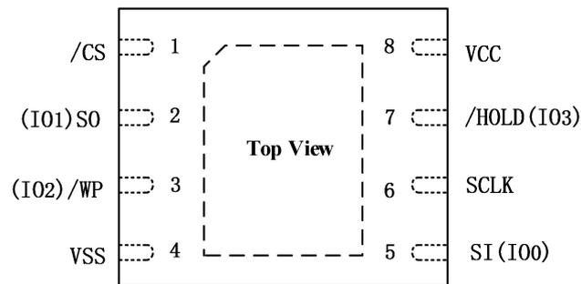
**Figure 3.2.** Pin Configuration USON8 4X3mm
