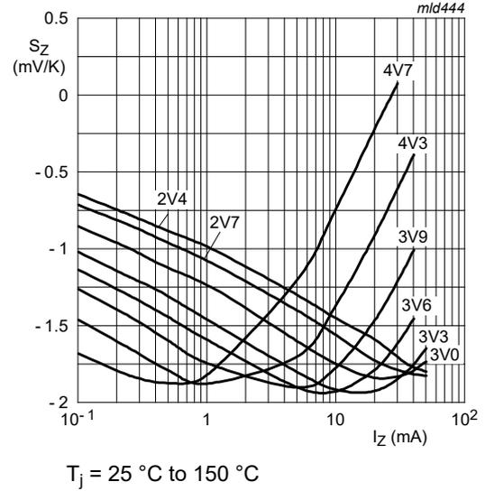
**Fig. 6. Temperature coefficient as a function of working current; typical values (BZX585-B/C2V4 to B/C4V7)**
