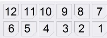
Control and monitor connector J4 (pin assignment is on left) is Molex Micro-Fit p/n 43045-1200. Mating connector is Molex Micro-Fit p/n 43025-1200 with crimp pins Molex p/n 43030-0009. Mating connector and necessary number of crimp pins are included with C151 Laser controller. Molex suggested crimping tool p/n 63819-0000 which can be purchased from Digikey Inc ([www.digikey.com](http://www.digikey.com))
