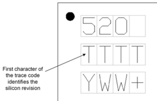
Figure 20.3. Device Package—DFN 10
