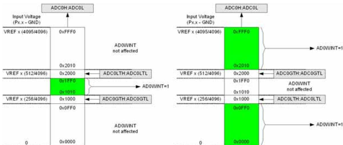
Figure 4.8. ADC Window Compare Example: Left-Justified Single-Ended Data
