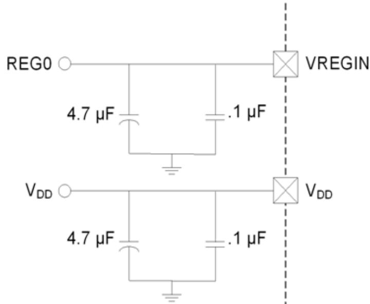
Figure 6.1. External Capacitors for Voltage Regulator Input/Output
