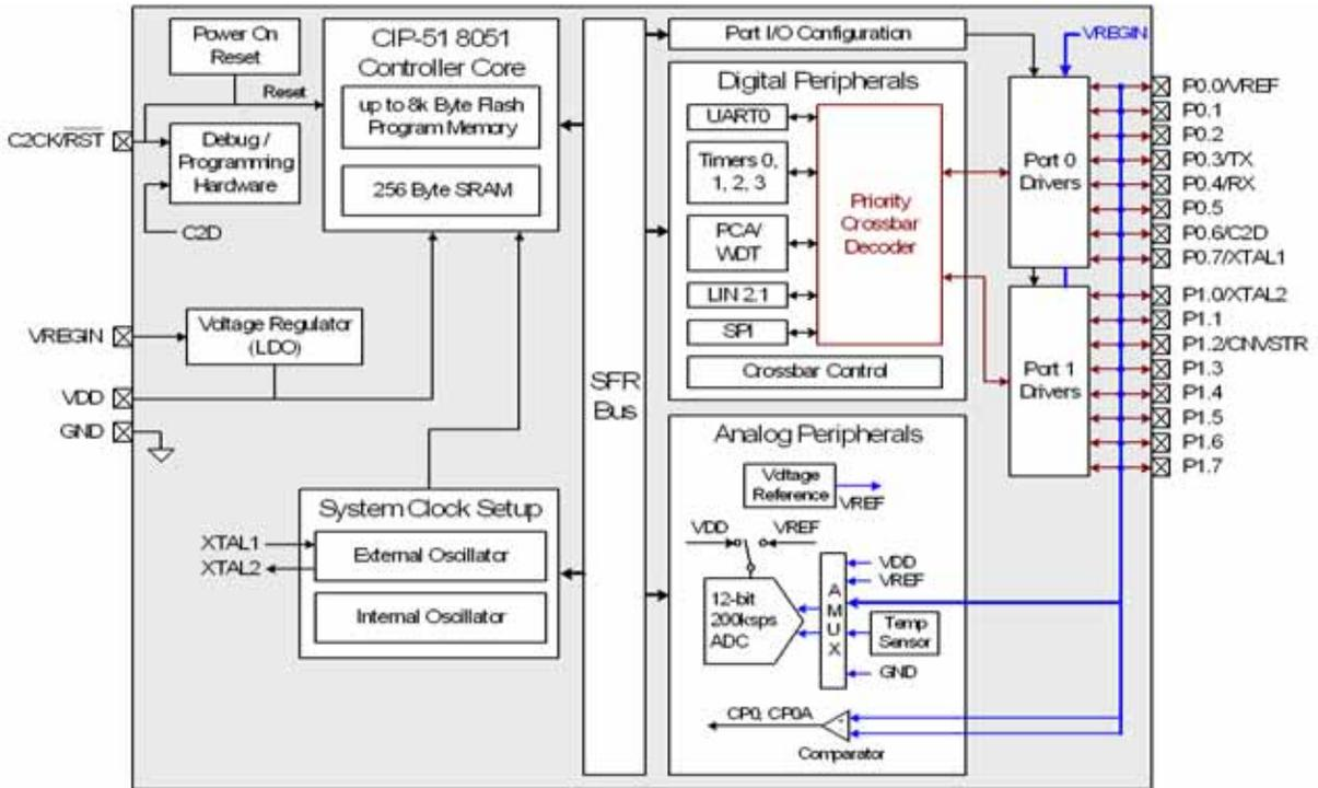
Figure 1.3. C8051F53x Block Diagram (Silicon Revision A)
