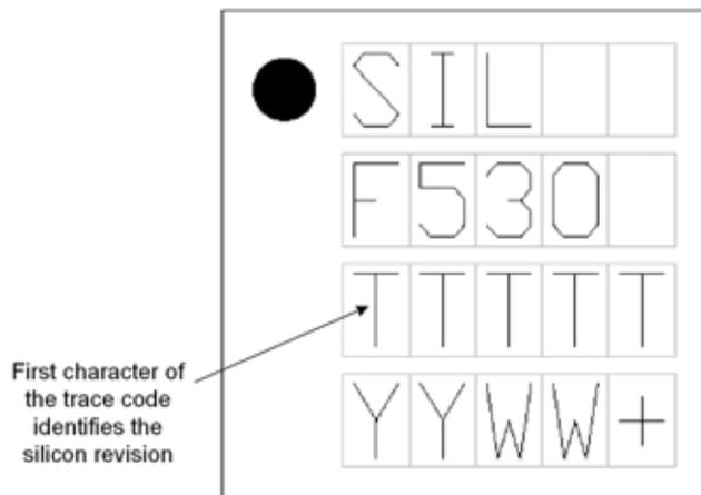
Figure 20.2. Device Package—QFN 20
