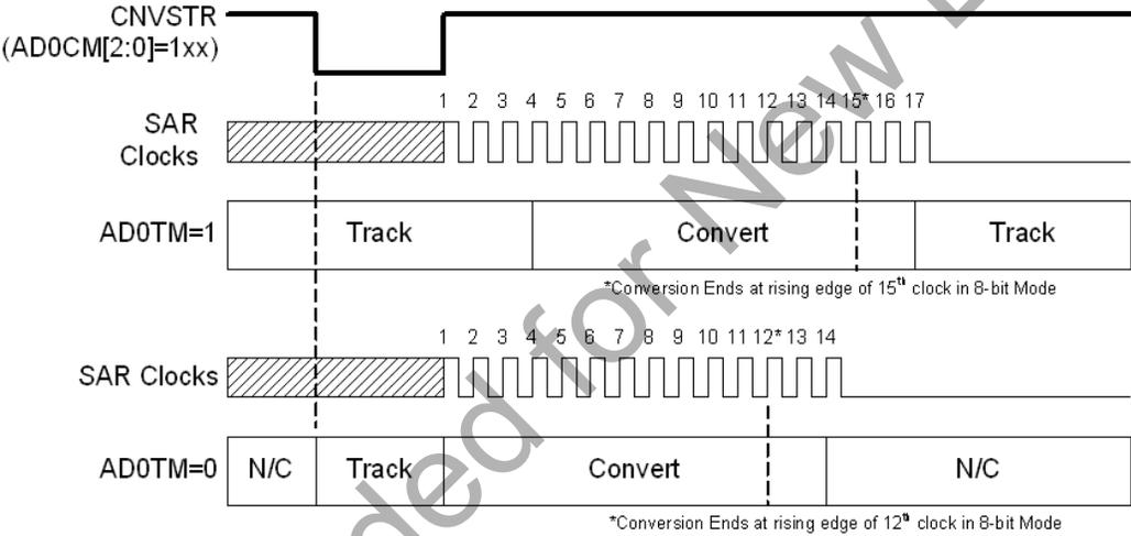
B. ADC Timing for Internal Trigger Source
