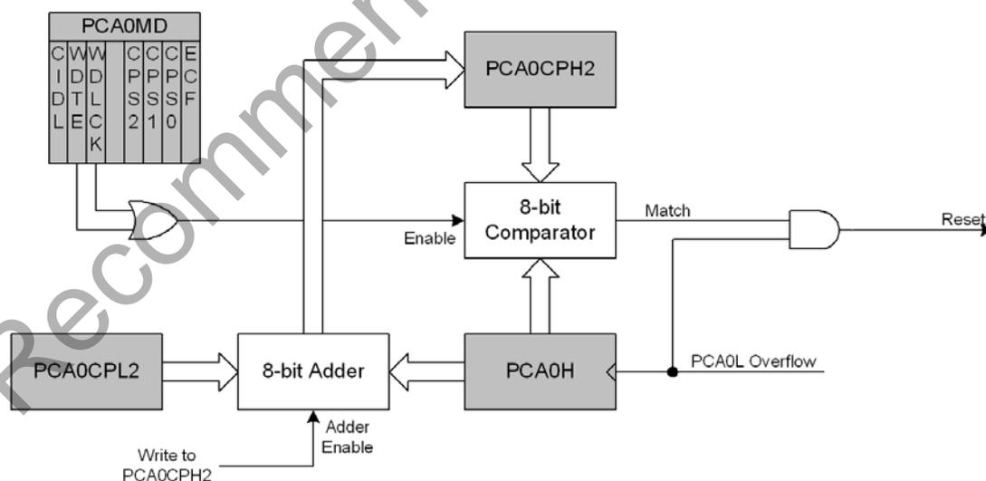
**Figure 29.11. PCA Module 2 with Watchdog Timer Enabled**
