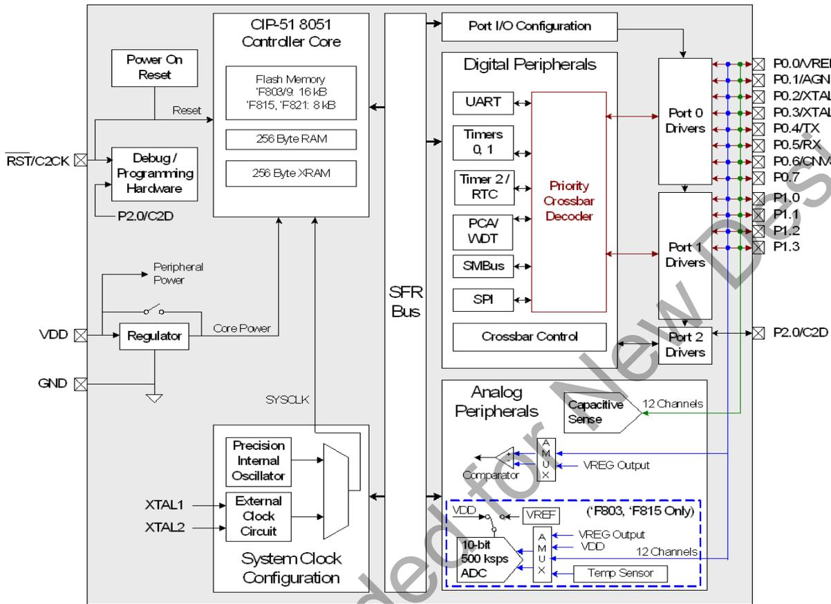
Figure 1.4. C8051F803, C8051F809, C8051F815, C8051F821 Block Diagram
