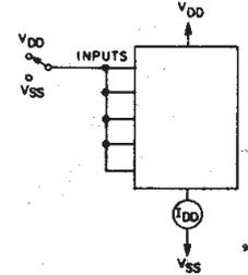
Fig. 13 - Quiescent device current test circuit.
