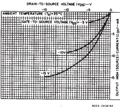
Fig. 5 - Minimum output high (source) current characteristics.
