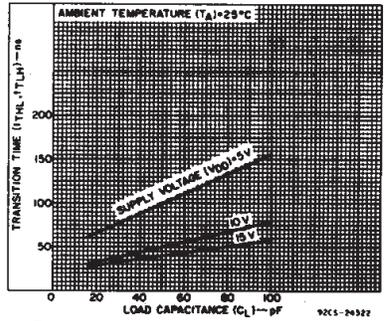
Fig. 11 - Typical transition time vs. load capacitance.
