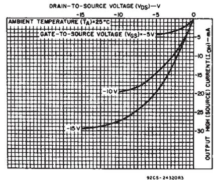
Fig. 4 - Typical output high (source) current characteristics.
