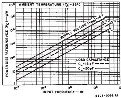
Fig. 10 - Typical power dissipation vs. frequency.
