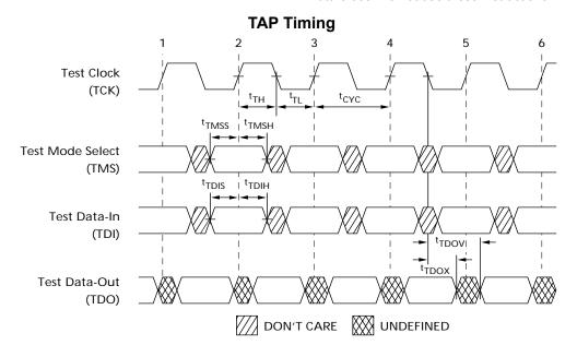
TAP AC Switching Characteristics Over the operating Range<sup>[10, 11]</sup>
