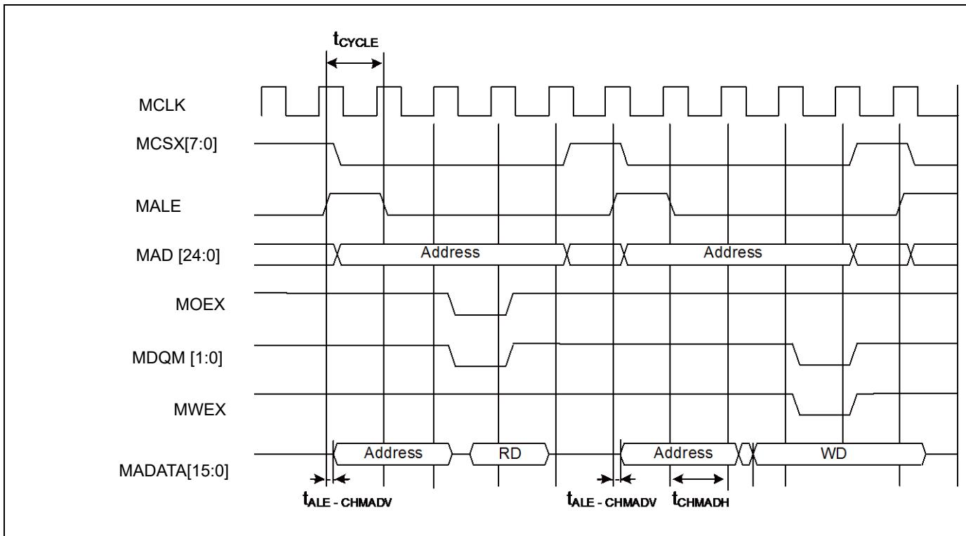
**Multiplexed Bus Access Synchronous SRAM Mode**
