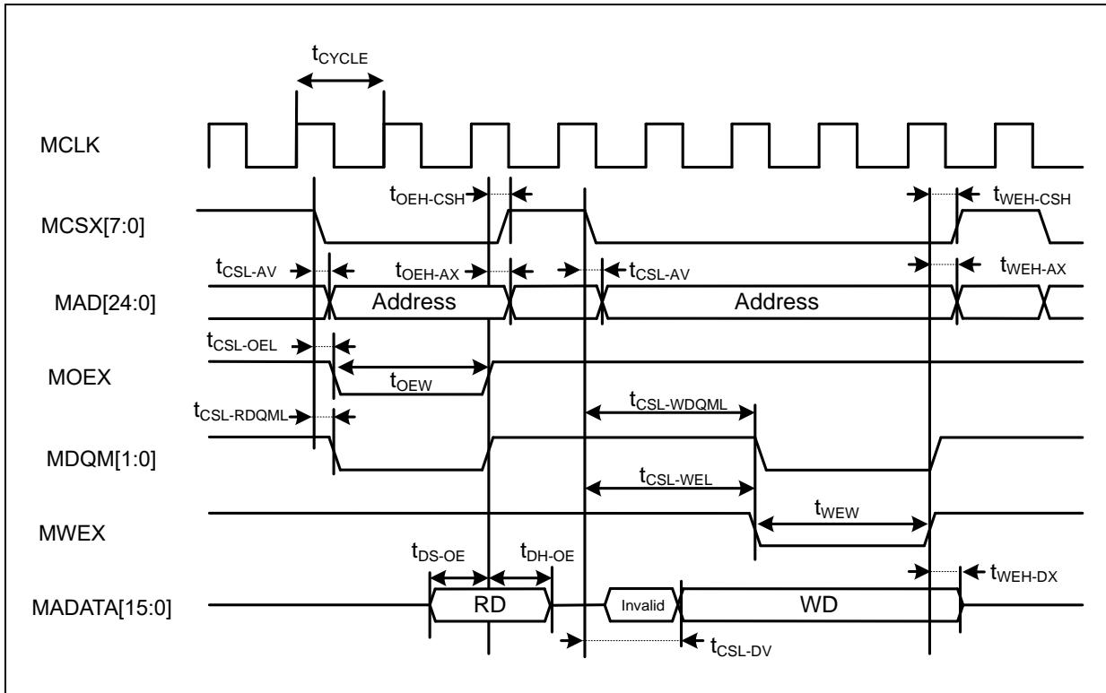
**Separate Bus Access Synchronous SRAM Mode**
