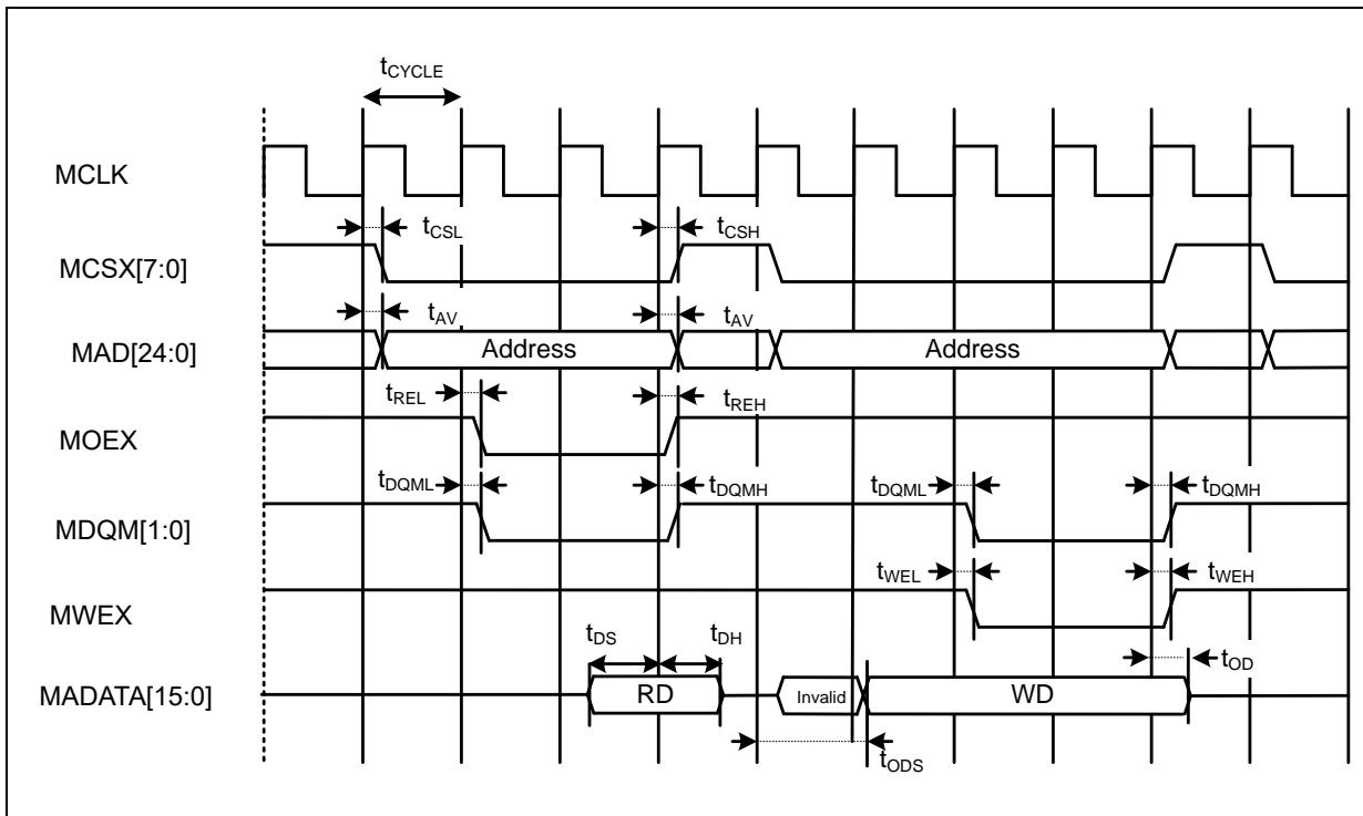
**Multiplexed Bus Access Asynchronous SRAM Mode**
