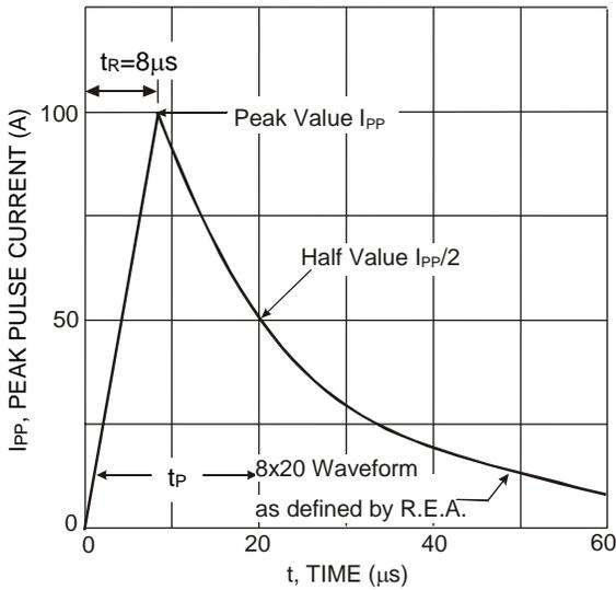
Figure 3 Pulse Waveform
