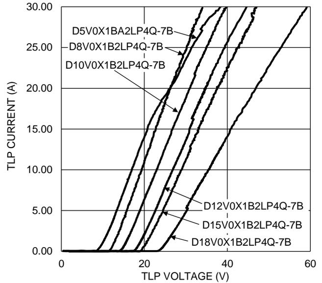
Figure 8 Transmission Line Pulse (TLP) Current vs. Voltage
