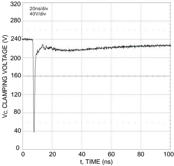
Figure 7 ESD Response to IEC 61000-4-2 (-8kV Contact Discharge)
