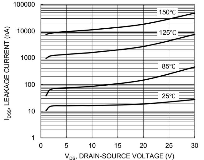
Figure 10. Typical Drain-Source Leakage Current vs. Voltage
