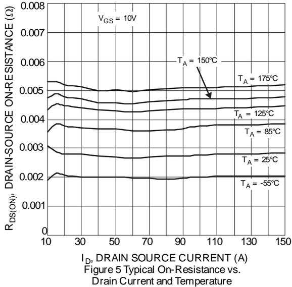
Figure 5 Typical On-Resistance vs. Drain Current and Temperature
